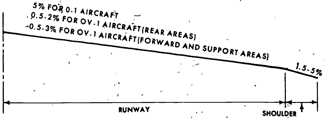
CENTER CROWN SECTION OF AIRFIELDS
