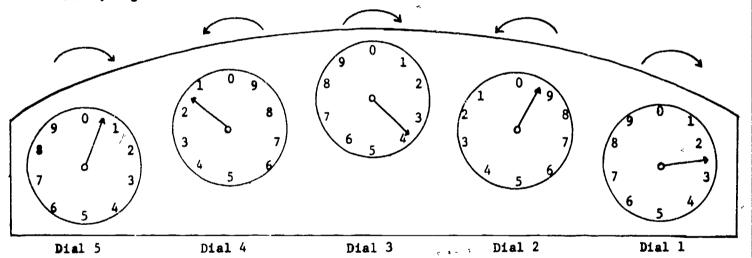
For example, to read the meter illustrated above, first notice that all the pointers do not turn in the same direction. The pointer on dial 1 (far right) is between 2 and 3, therefore, 2 is the figure to use and the reading so far is: ----2.
