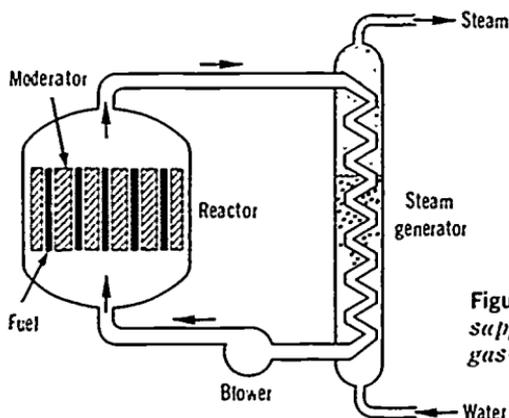
Figure 5 Nuclear steam-supply components in a gas-cooled reactor.
