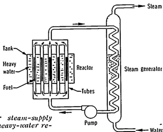
Figure 6 Nuclear steam-supply components in a heavy-water reactor.
