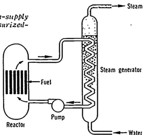
As you can see, a nuclear steam supply that uses a pressurized-water reactor consists of two separate water systems that meet in the steam generator. The water in one system does not mix with that in the other, but heat is transferred from the reactor system to the steam system.
