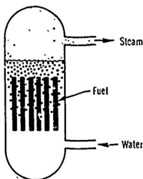
Figure 3 *Nuclear steam-supply components in a boiling-water reactor.*
