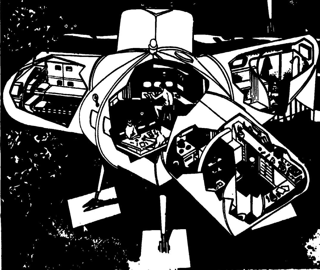
The DS-2 DIVING SAUCER. A mechanical claw tears specimens from the ocean floor, then drops them into a basket under the hull. It is one of the four units used in Conshelf 2 (see Starfish House below).
