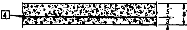
TYPICAL FLOOR SLAB UNDER MEDIUM WEIGHT MACHINES NOT TO EXCEED 300 PSF ASSEMBLY 1417
