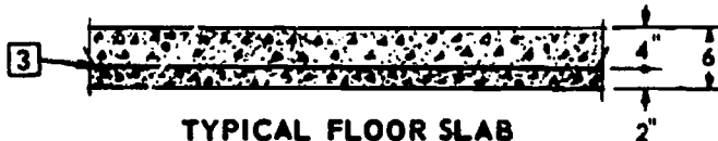
TYPICAL FLOOR SLAB UNDER LIGHT WEIGHT MACHINES NOT TO EXCEED 200 PSF ASSEMBLY 1416
