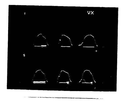
Fig. 16. Voicing-loudness-binary nasality composite display for a normal male speaker's two versions of the utterance "pne two three." Nasality criteria identical to those used in Figure 14.
