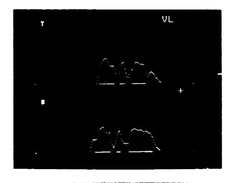
Fig. 12. Voicing-loudness composite display for a male speaker's utterances of two 3-syllable words. Top: "destitute"; bottom: "testify." Note breaks in the loudness function caused by total vocal-tract closure for the three medial occurrences of the /t/ in the two words.
