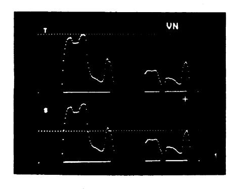
Fig. 13. Voicing-nasality composite display for a normal male speaker's utterance of "Monday" and "Tuesday." Data from the lower half of the display have been copied to the upper half under user control.
