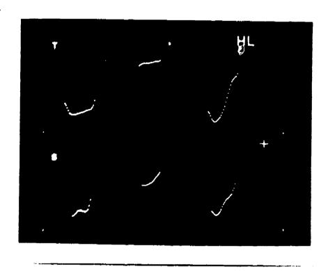
Fig. 8. High-low function display for six words spoken by a male. Left to right; top to bottom: "sod, seed, side"; "bought, boot, bout."
