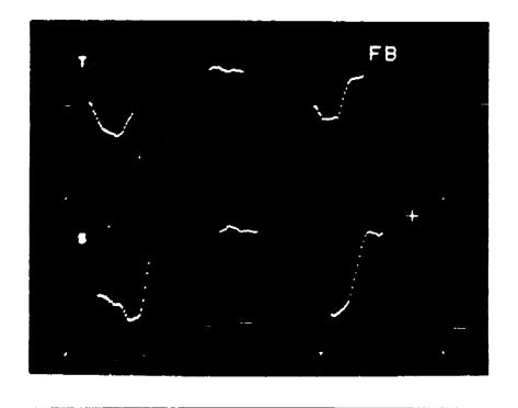
Fig. 9. Front-back vowel function display for six words spoken by a male. Left to right; top to bottom: "Sod, seed, side"; "pose, peas, poise."
