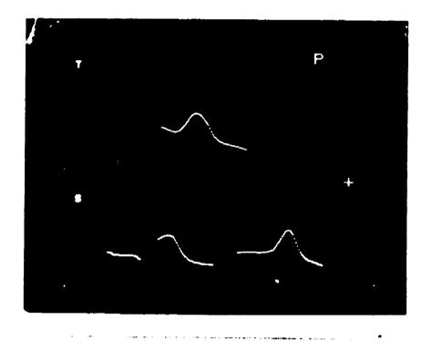
Fig. 7. Pitch display for two utterances produced by the same male speaker. Top trace: "Now are you?" Bottom trace: "I'm fine. Now are you?"
