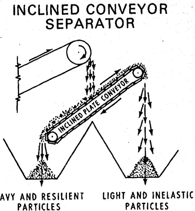
Figure 4. Types of inertial separators.
