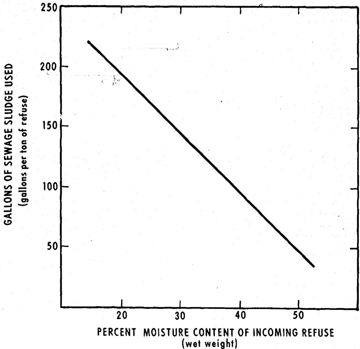
Figure 3. The amount of sewage sludge (gallons) at 3 percent solids that can be used without dewatering varies in direct proportion to the moisture content of the incoming refuse. Actual amount of refuse ground and mixed with sludge would be 75 percent of that received. These proportions would result in a mixture containing 60 percent water by wet weight.
