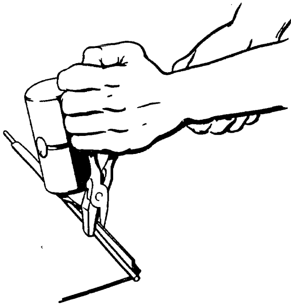
AM.283 Figure 5-41.—Hand forming a wire edge.
