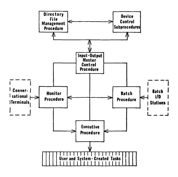
Figure 2. Major System Procedures and Their Lines of Communication
