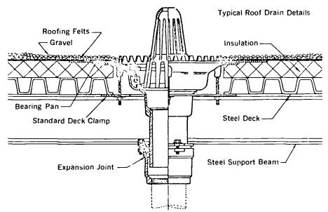
Roof drain shown installed in a steel deck in combination with the expansion joint. Note that the use of the bearing pan insures a recessed drain at the leader. The expansion joint absorbs deck contraction and deflection.
