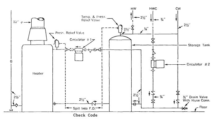
Fig. 10-1 Typical Water Heater Piping
