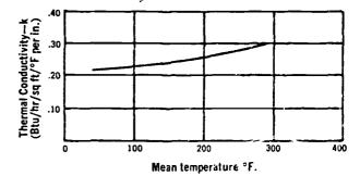
Fig. 18-1 Fiber Glass Insulation
