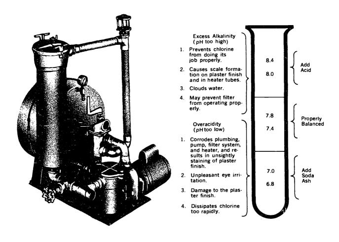
Fig. 16-4 Preassembled Filter Assembly
