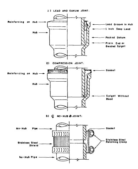
Fig. 6-2-The Various Joints Presently Being Used to Connect Cast Iron Soil Pipe and Fittings
