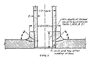
FIG. 13(F) WELDED-ON TAPPED PAD.
