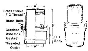
Fig. 15-2 Roof Drain Details
