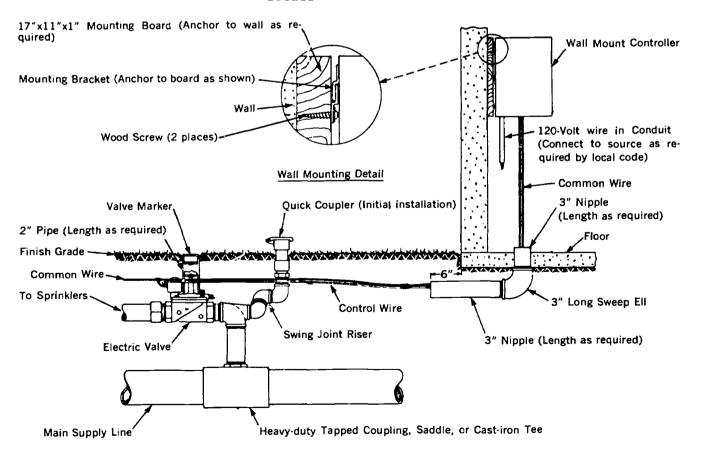
Fig. 16-13 Typical Electric Controller & Valve Assembly Detail
