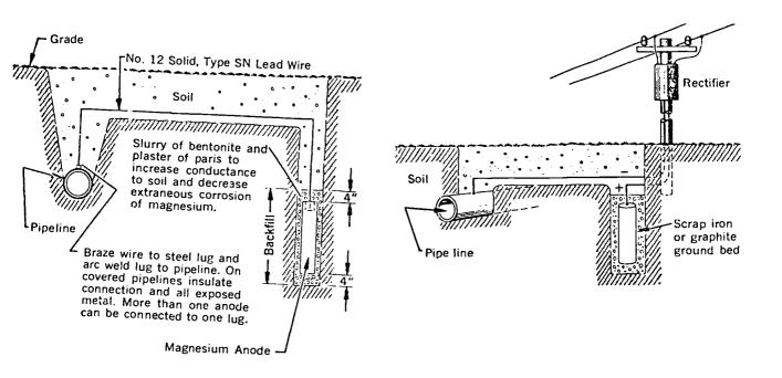
Fig. 17-1 Cathodic Protection
