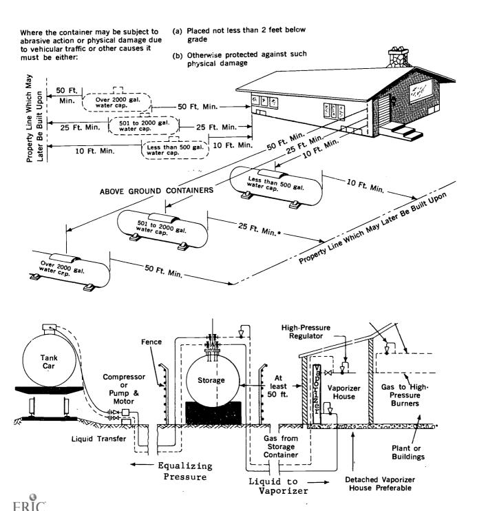
Fig. 12-1 L-P Gas Installation Details
