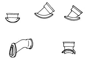
Building sewers are connected to public sewers by means of sewer saddles which fit over or into a hole tapped in the pipe (clay, concrete, asbestos cement, fiber). The saddle is usually held in place by cement.
