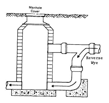
Fig. 7-2 Manhole Detail
