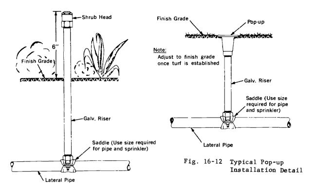
Fig. 16-11 Typical Shrub Head Installation Detail
