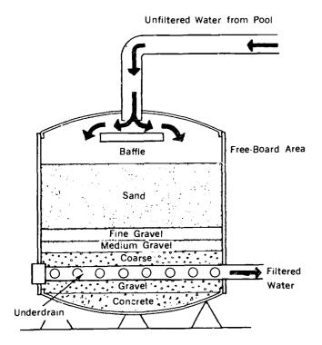
The filtering process starts with the delivery of pool water to the top of the filter tank. The water is pressure-forced through descending layers of sand and fine, medium, and coarse gravel, and then—filtering completed—it is collected in a perforated pipe (underdrain) and returned to the pool.
