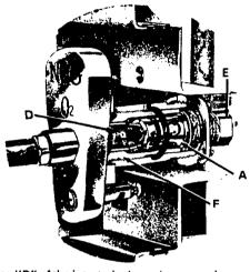
Nose "D" of the inserted adapter has moved poppet "A inward, through O-Ring seal, and gas flows through the adapter. Leakproof seal of adapter is accomplished around the O-Ring encircling the barrel. Marring and nicking of adapter nose does not minimize effectiveness since the adapter is *not* of nose seating design.
