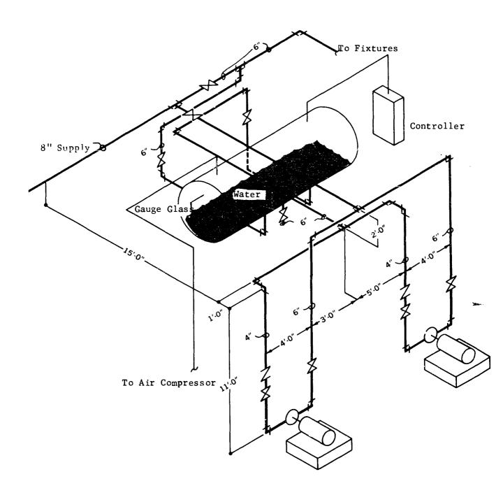
Fig. 10-3 Typical Hydropneumatic Water Pressure System
