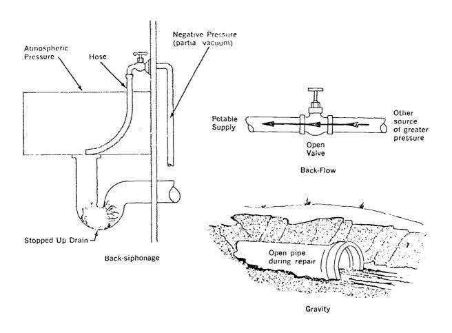
Fig. 10-8 Methods of Contamination
