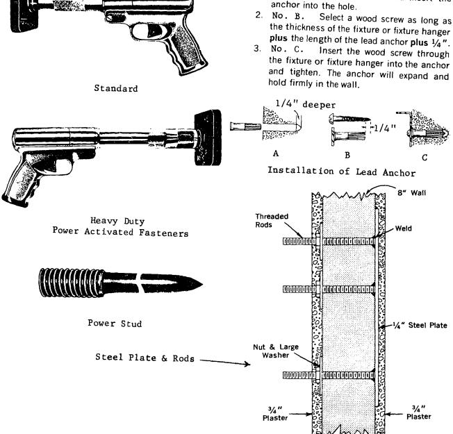
Fig. 5-1 Types of Fasteners
