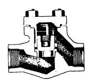
Globe Type Lift Check Valve Courtesy- Crane Co.
