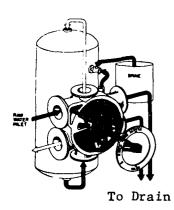
Regeneration—Raw water enters valve, draws in brine, flows down through the bed to bottom of tank, returns to valve and out to drain.
