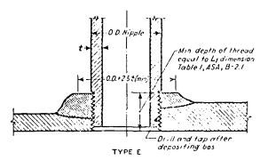
FIG. 13(E) BUILT-UP WELDED TAMPED BOSS
