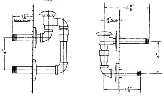
Fig. 10-9 Vacuum Breakers
