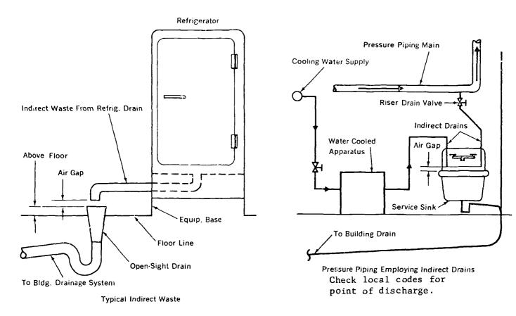
Fig. 9-3 Indirect Drains
