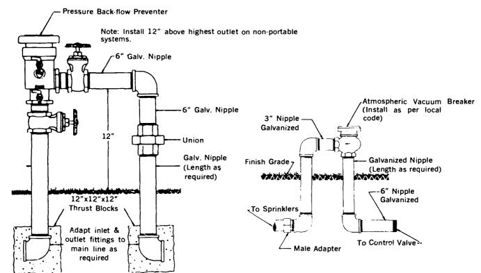
Fig. 16-8 Typical Back-flow Preventer
