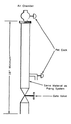
An air chamber is a section of water piping on which the upper end is closed, and the lower end is connected to the piping system. On horizontal piping, it is connected by means of a side outlet tee; on risers and water supply branches, it is installed at the top.
