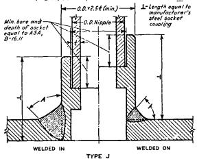
FIG. 13(J) WELDED FULL SOCKET COUPLING
