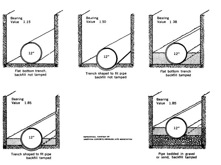
Fig. 7-1 Methods of Bedding Pipe and Bearing Values
