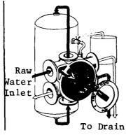
Rinsing—Raw water enters valve, flows from top of tank to bottom where water is directed through valve to drain.
