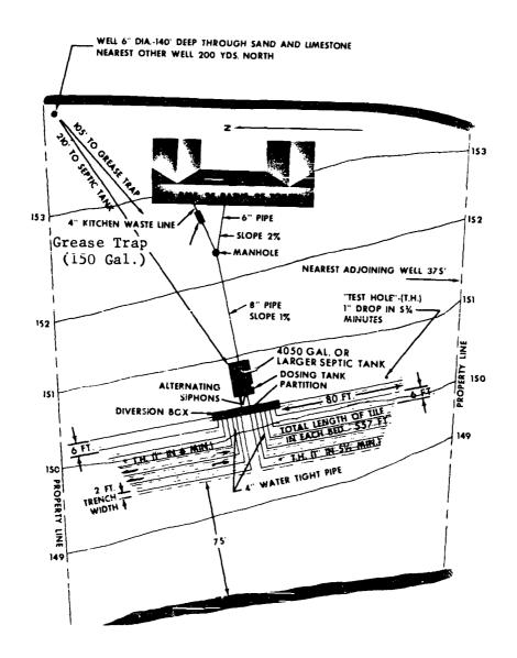
Fig. 8-1 Typical Leaching Field Layout Check Local Code
