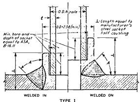
FIG. 13(1) WELDED HALF SOCKET COUPLING.
