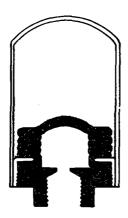
1. Before installation, the bellows are held in a full compressed position by pressurized gas in the upper part of the chamber,
