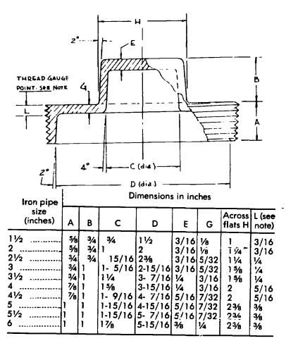
Note—When thread gauge is screwed tightly on plug by hand, large end of gauge shall be the distance "L"  $\pm 1\,1/2$  turns, from surface of plug.
