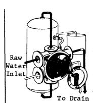
Backwash—Raw water enters valve, flows from bottom of tank to top, return to valve and out to drain.
