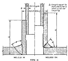
FIG. 13(H) WELDED FULL TAPPED COUPLING
