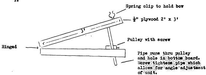
Unit sits on table top outside - we use large park-ground picnic tables, which are very solid. Masking tape is placed on top board and marked with standard unit to measure DRAW.
