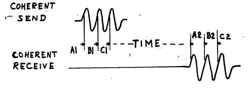
Figure 4. Noncoherent versus coherent ranging.
