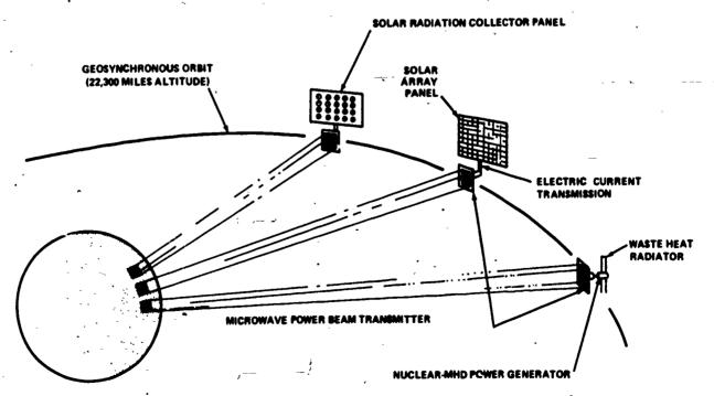
Figure 3. Methods of power generation in space for consumption on earth.
