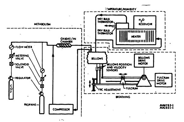
Figure 1. BMS subsystems.
