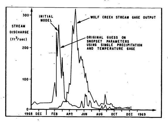
Figure 5. Calibration of hydrological model parameter for Wolf Creek Drainage Basin.
