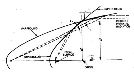
Figure 8. Two reflections from a paraboloid and hyperboloid of resolution.
