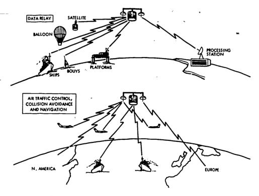
Figure 7. Satellite systems for data relay and navigation.
