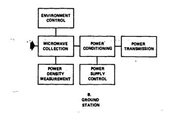
Figure 3. Major components of a satellite solar power station.
