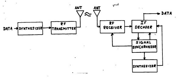
Figure 5. A simplified FH system with synthesizers.
