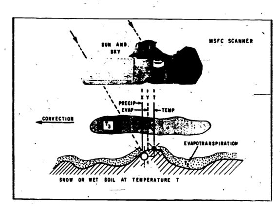
Figure 9. Precipitation estimates from change of water vapor and temperature maps.
