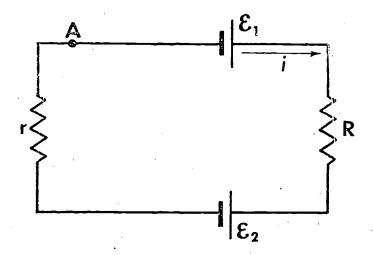
12 (30-23). Find the current in the 1-ohm resistor in the circuit shown below.
