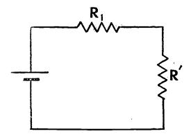
we see that  $R_1$  and R' are connected in series, so the equivalent resistance of the emuire circuit, R, is
