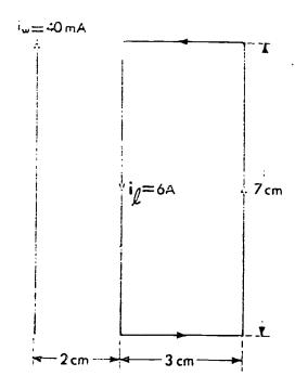
We utilize the symmetry of the configuration to reason that the forces on the two short sides of the loop are equal and opposite and will add to zero. The force on the near side of the loop is repulsive (anti-parallel currents). Its magnitude is
