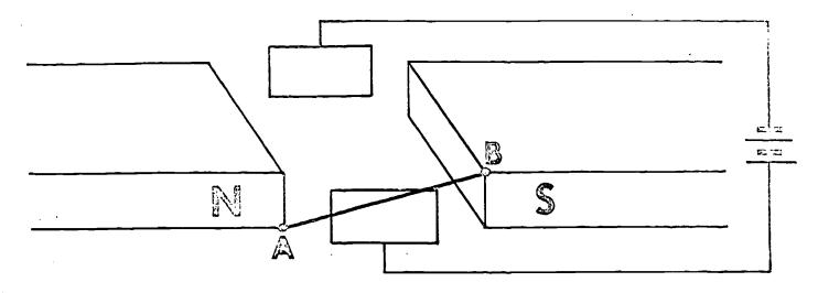
The above figure shows crossed electric and magnetic fields. The electric field intensity is 100 nt/coul, the magnetic induction is 2 T. A particle enters the field from below and travels along a line parallel to the line AB. This path makes an angle of 30° with the horizontal. With what speed must the particle move to remain undeflected in its path?
