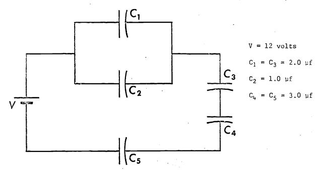
10 (26-15). In the diagram below, what fraction of the total charge will be on one plate of the capacitor  ${\rm C_2}$ ?
