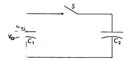
13.(27-10). Two identical capacitors have their plates initially separated by a layer of air. A sheet of mica ( $\kappa = 8$ ) is then inserted into the air space of the second capacitor, completely filling it. What is the ratio of the capacitance without dielectric to that of the other; namely,  $C_a/C_d$ ?
