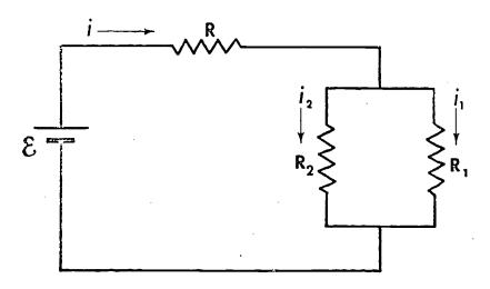
11 (30-19). Write the loop equation for the circuit shown below. Assume that current i flows clockwise through the circuit.
