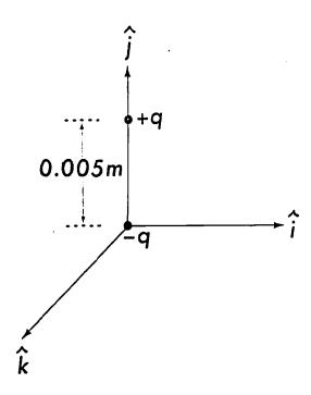
An electric dipole, consisting of opposite charges each of magnitude  $3.2\times10^{-19}$  coul, is arranged as shown in the above diagram. What is the magnitude and direction of the dipole moment?
