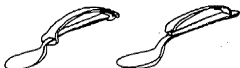
Strap of leather or rubber over back of hand Metal bar for palmar
