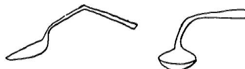
Bent handle for flexion, extension difficulty Bent handle for pronation, supination difficulty
