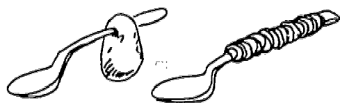
Padding for stability in conventional grasp Handle weighted with solder
