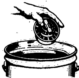
Oil Fill Cap with Filter Element: Clean and lightly re-oil. Replace cap if filter element is clogged.
