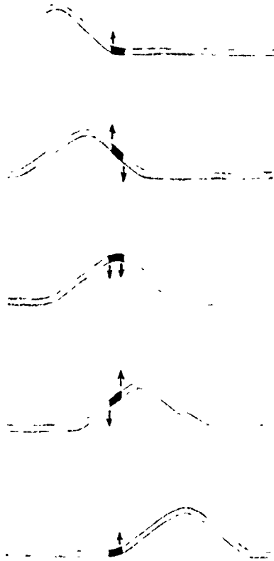
Fig. 12.5 A rough representation of the forces on a small section of rope as a transverse pulse moves past it.
