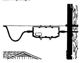
Performance standa · Js limit the number of amplifiers that can be connected in line on one coaxial cable to about 25 trunk amplifiers, spaced 2.8 amplifiers per mile of 3/4-inch cable. This rule of thumb implies that trunk lines cannot extend more than approximately eight miles from each headend without unacceptable loss of signal quality.
