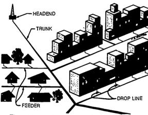
The cable that leaves the headend, called the trunk line, is about one-half to three-quarters of an inch in diameter. To distribute the cable to subscribers' homes, the trunk line is connected to smaller feeder lines. Finally, individual drop lines run into each household.
