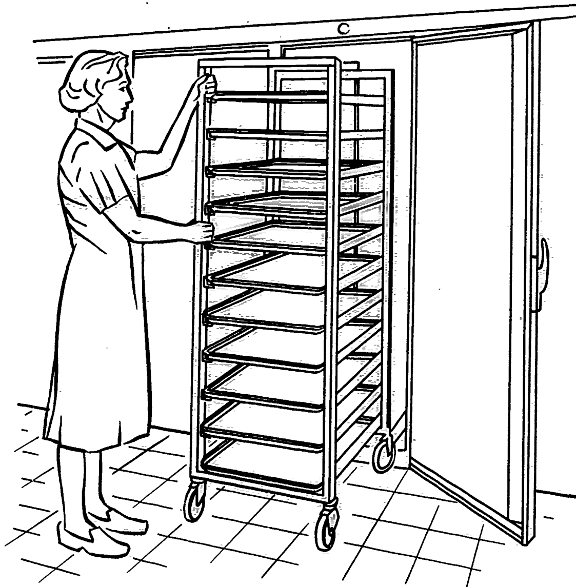
FIGURE 21.—Portable tray rack for use in walk-in refrigerators.
