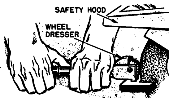
Figure 10-4.—Using a grinding wheel dresser.
