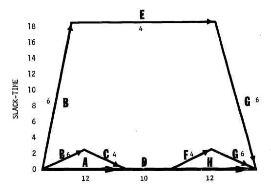
The same holds true for the FG path H - (F + G). The BEG path has 18 days slack time, (A + D + H) - (B + E + G). Neither B or G can be delayed more than 2 days each because of their A and H relationship. This means that activity E could plan to be delayed at least 18 - (2 + 2) or 14 days at normal-time and not hold up the total job.
