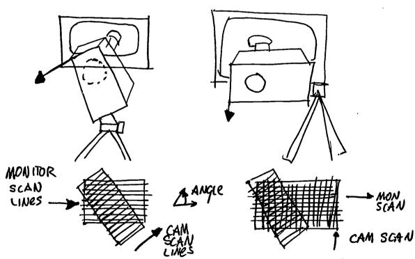
(OF COURSETHE DISTANCE IS EQUIVALENT TO A TIME INTERVAL BETWEEN CAMERA AND MONITOR SCAN POINTS)
