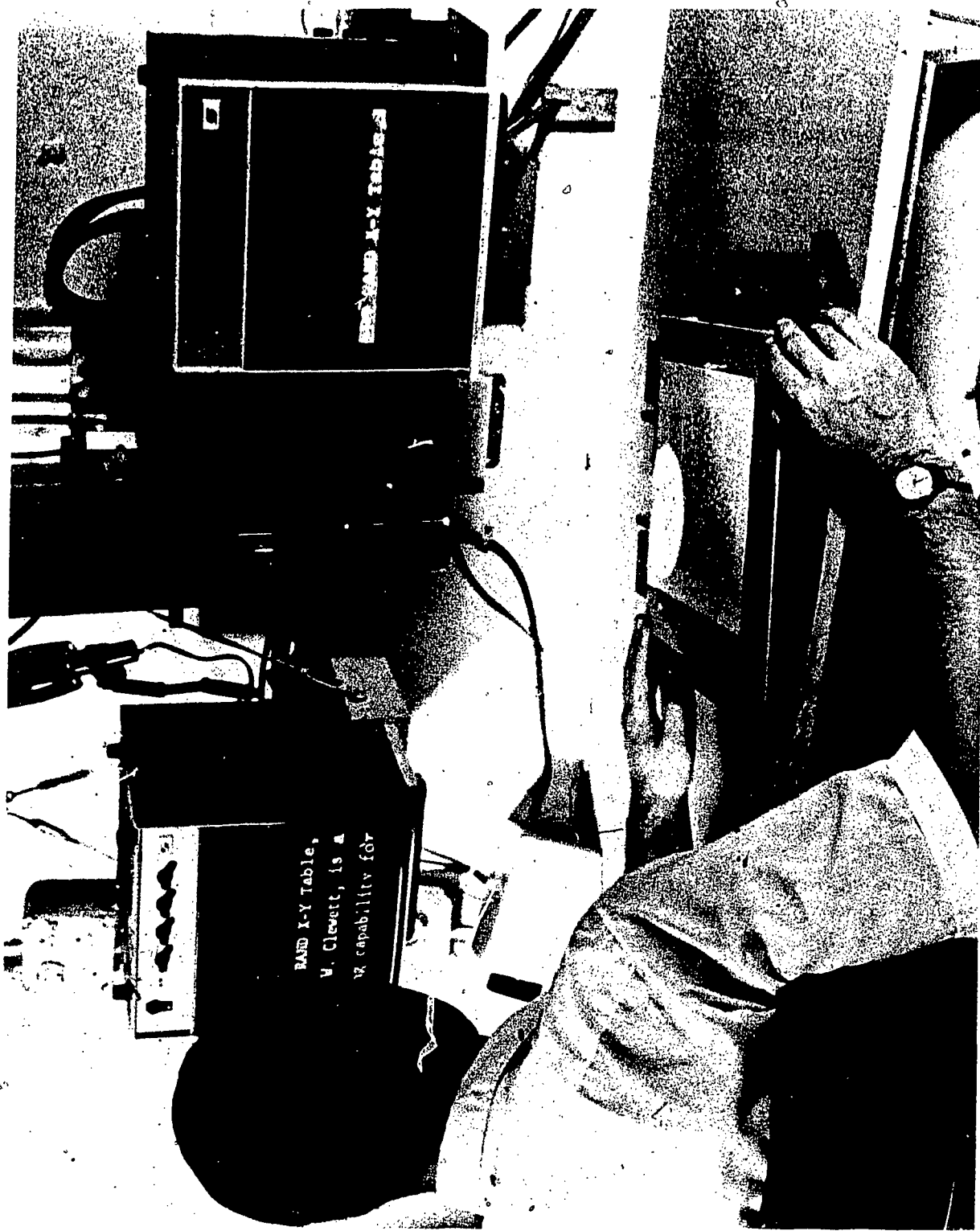
Fig. 10—X-Y Platform being used for reading in conjunction with RANDSIGHT I
