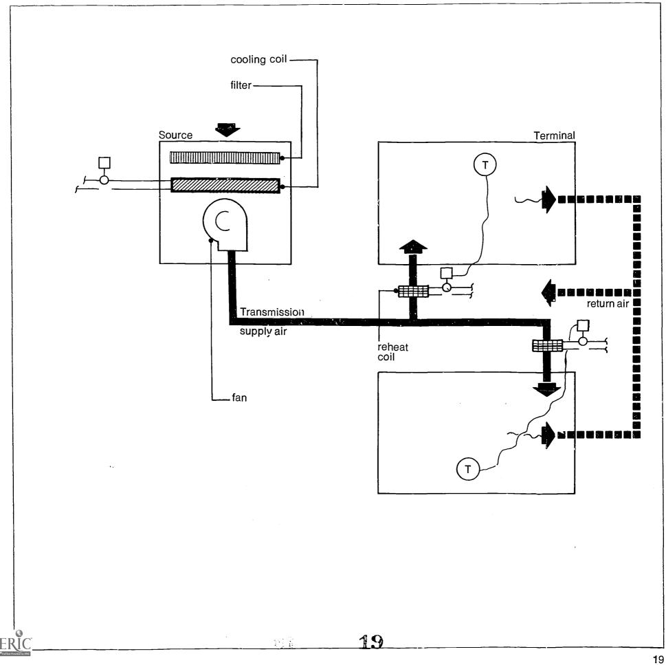
Figure 11: Single-duct induction unit (air and water system)
