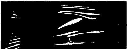
(c) Representative smoke pictures showing smooth and turbulent flow over airfoil.
