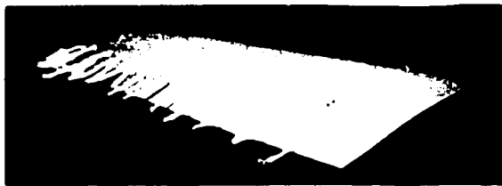
(c) Representative smoke pictures showing smooth and turbulent flow over airfoil.
