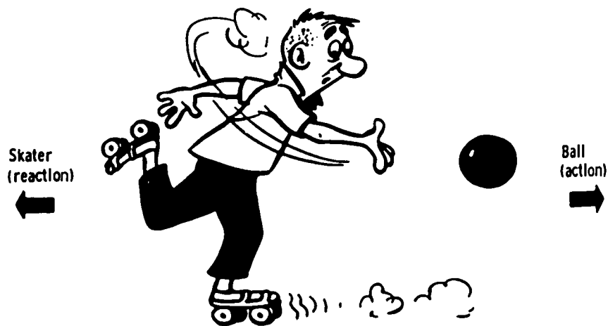
Figure 2-2. - Newton's Third Law of Motion. Reaction - For every acting force there is always an equal and opposite reacting force.
