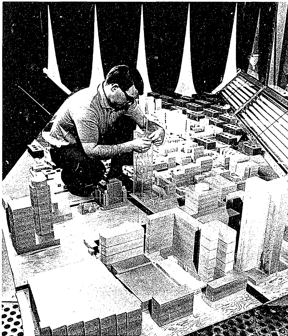
Low speed aeronautical wind tunnel modified by spires to create a turbulent shear flow simulating surface winds over model of downtown Montreal. Instrumented plexiglas model of a 600 ft. office building, on which full-scale pressure measurements have been taken, in centre. A cooperative project of Division of Building Research and National Aeronautical Establishment.
