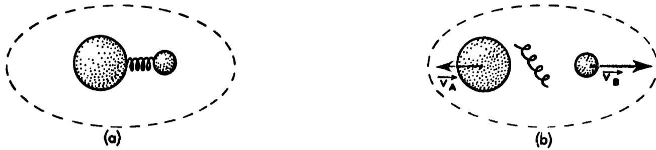
Fig. 2.1 The system of two spheres and a small spring. That the system is isolated is schematically indicated with an imaginary dotted line.
