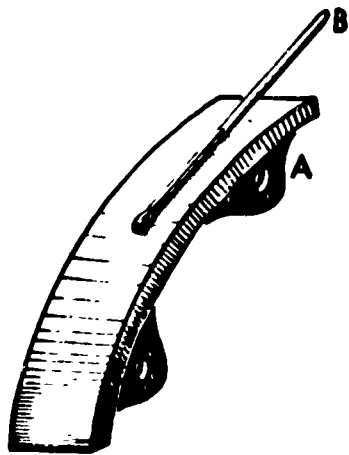
Fig. 3.3 Brake shoe A and thermometer B in physical contact. The brake shoe and the thermometer are at the same temperature when there is no net energy flow into or out of the thermometer, as demonstrated by the fact that the length of the liquid in the capillary tube does not change with time.
