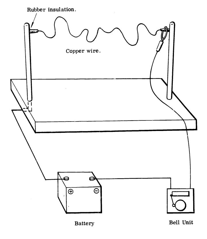
The loop should be passed along the wire without touching it. If the loop touches the wire the bell will ring.
