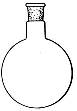
Mark shank of B14 socket to appropriate length allowing for thickening of glass. For blowing bulb - seal off to length, melt, thicken and form flask to size.
