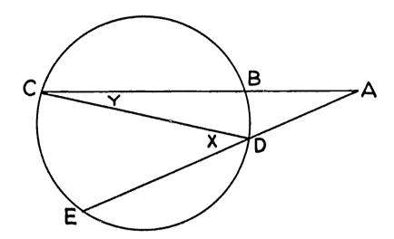
Then the number of degrees in arc CE is 2x and in arc DB is 2y. But the number of degrees in  $\angle A$  is (x - y). Therefore an angle formed by two secants intersecting outside the circle is measured by one half the difference of the intercepted arcs.
