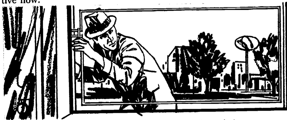
Intruders can easily defeat metallic foil on windows by cutting glass as illustrated. See next page.
