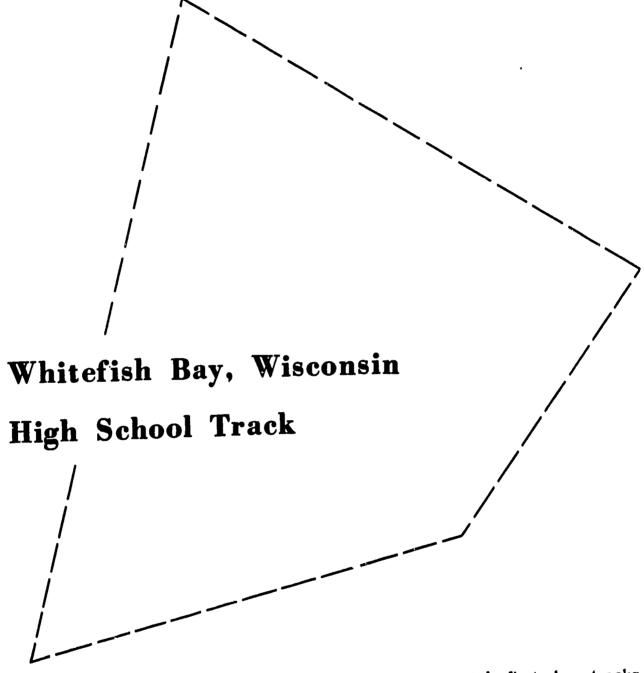
The Whitefish Bay High School track is one of Wisconsin's first-class tracks. It is a full quarter-mile in circumference with a 230-yard straightway, 27 feet wide, on the east side. The track is 17 feet wide on both curves and on the backstretch. The curves have a radius of 117 feet.
