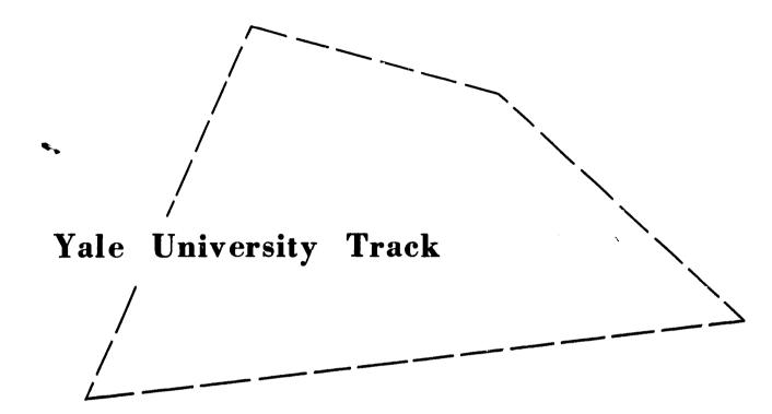
The Yale University track is a full quarter-mile with two 260-yard straightaway sides extended from the oval. The radius at the curb is 90 feet, making a full circular arc. The track is 25 feet wide and 3 feet deep. To construct it, a deep layer of brush wood was covered with a layer of large rock, and then with afootbed of coarse clinkers. The final cover of 8 inches was made of a mixture of *bead-on clinkers*, clay, and loam.
