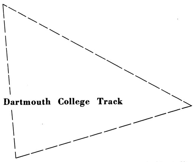
The Dartmouth College track is constructed on a radius of 106 feet. Its 220foot straightaway is 24 feet wide, and its curves and back stretch are 20 feet wide. The cement curb is 24 inches in depth with a widened bottom to prevent heaving from frost.
