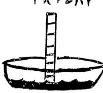
Observe and measure each pan with ruler or other measuring device to record evaporation.
