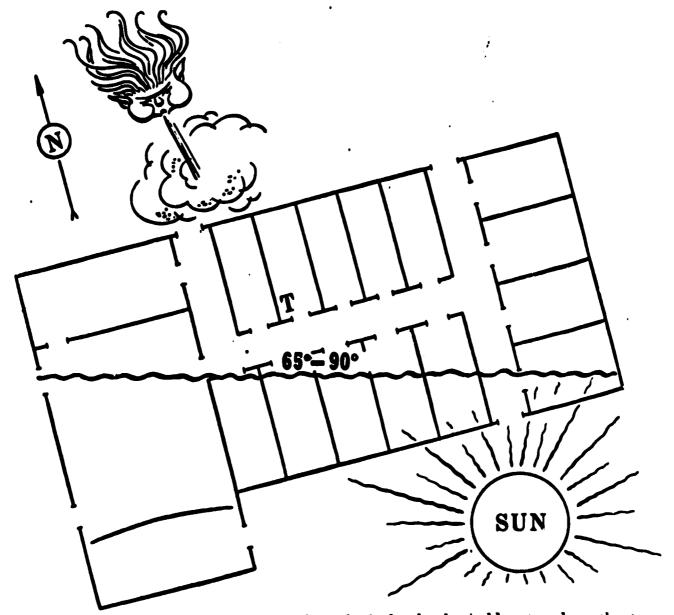
One control (T) in this hypothetical school would not reduce the temperature range to which students would have to adjust. If the entire school were placed under this one control, the control would have to be set at a "high" figure so that the other classrooms would have at least "average" temperature.
