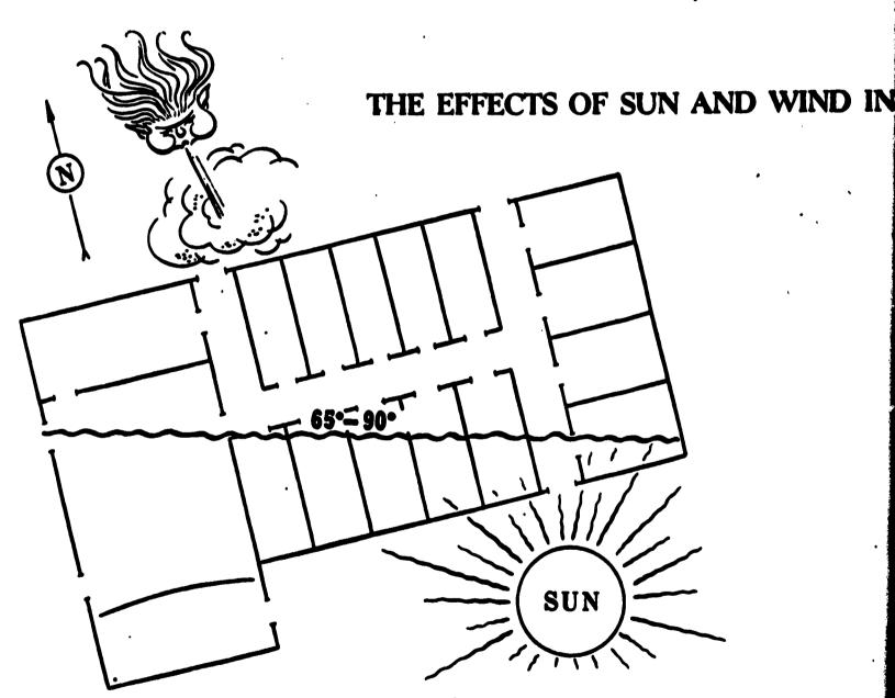
Sun and wind are dynamic factors in classroom heating and ventilating. Here, in this hypothetical school, the sun and wind have created a 25-degree temperature differential. Thermal conditions in each classroom will change as the sun moves, as the wind shifts, increases or decreases.
