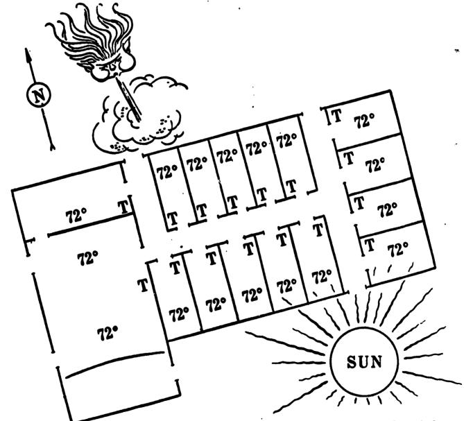
The only positive solution to thermal disturbances caused by wind, sun and the other dynamic heat factors is a system of individual room controls. Students can move freely within the classroom, and from classroom to classroom, with a minimum of adjustment. Savings in physical and nervous energy can be applied directly in biological and growth processes or in classroom tasks.
