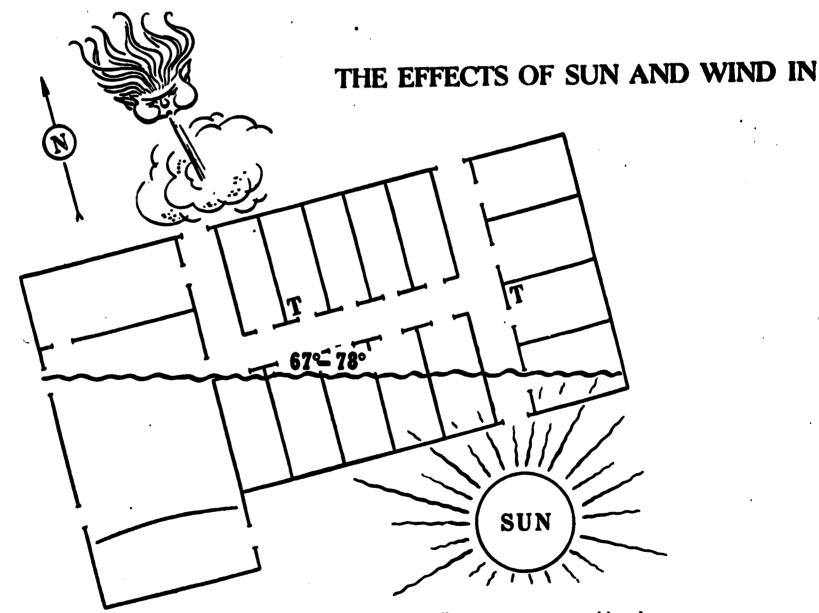
Two controls (T)—in a modified "zoning" arrangement—would reduce the range of temperatures in a school to about half. Temperature adjustments would still be at least 10° F. Zone systems are unable to compensate for changes which have their origin in the classroom, such as the size of the class or the type of class activity.
