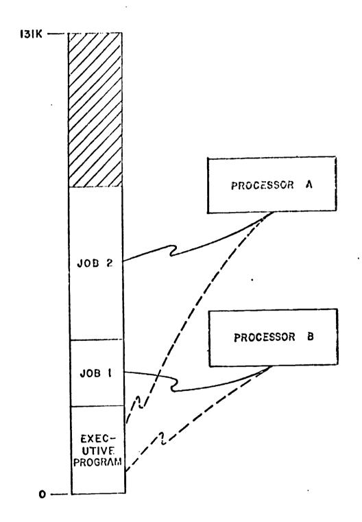
Fig. 2: Multiprocessing System (without Multiprogramming)
