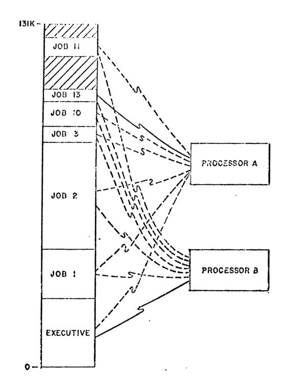
Fig. 4: Multiprogramming-Multiprocessing System
