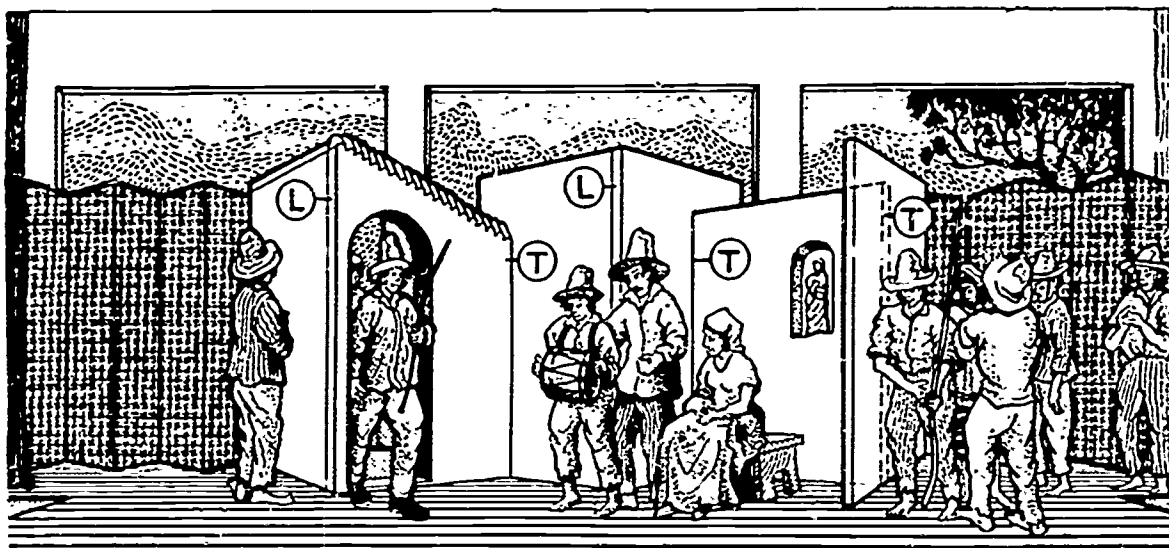
Illustration 8: The designer must arrange for groupings of panels using the maximum number of "L" and "T" joints.
