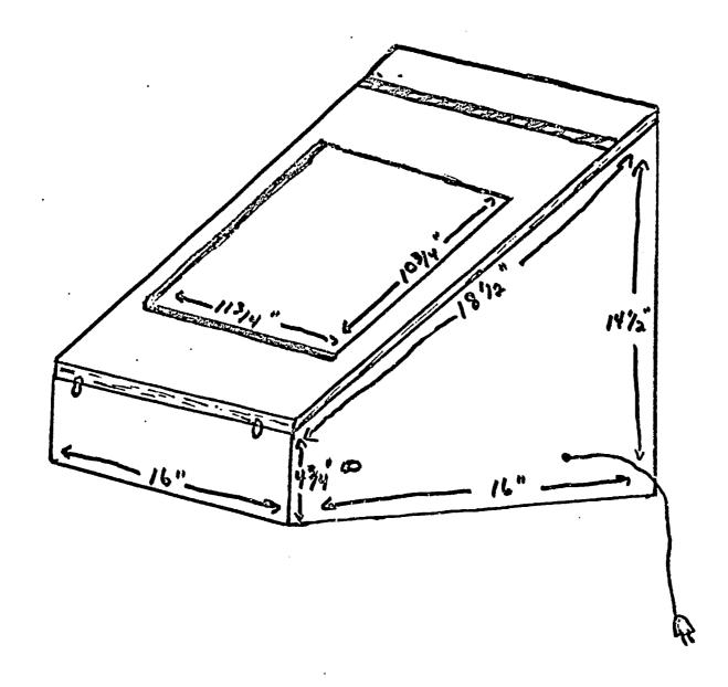
A pane of frosted glass is set into the top of the light box and edged at the left and bottom by a perpendicular flange.
