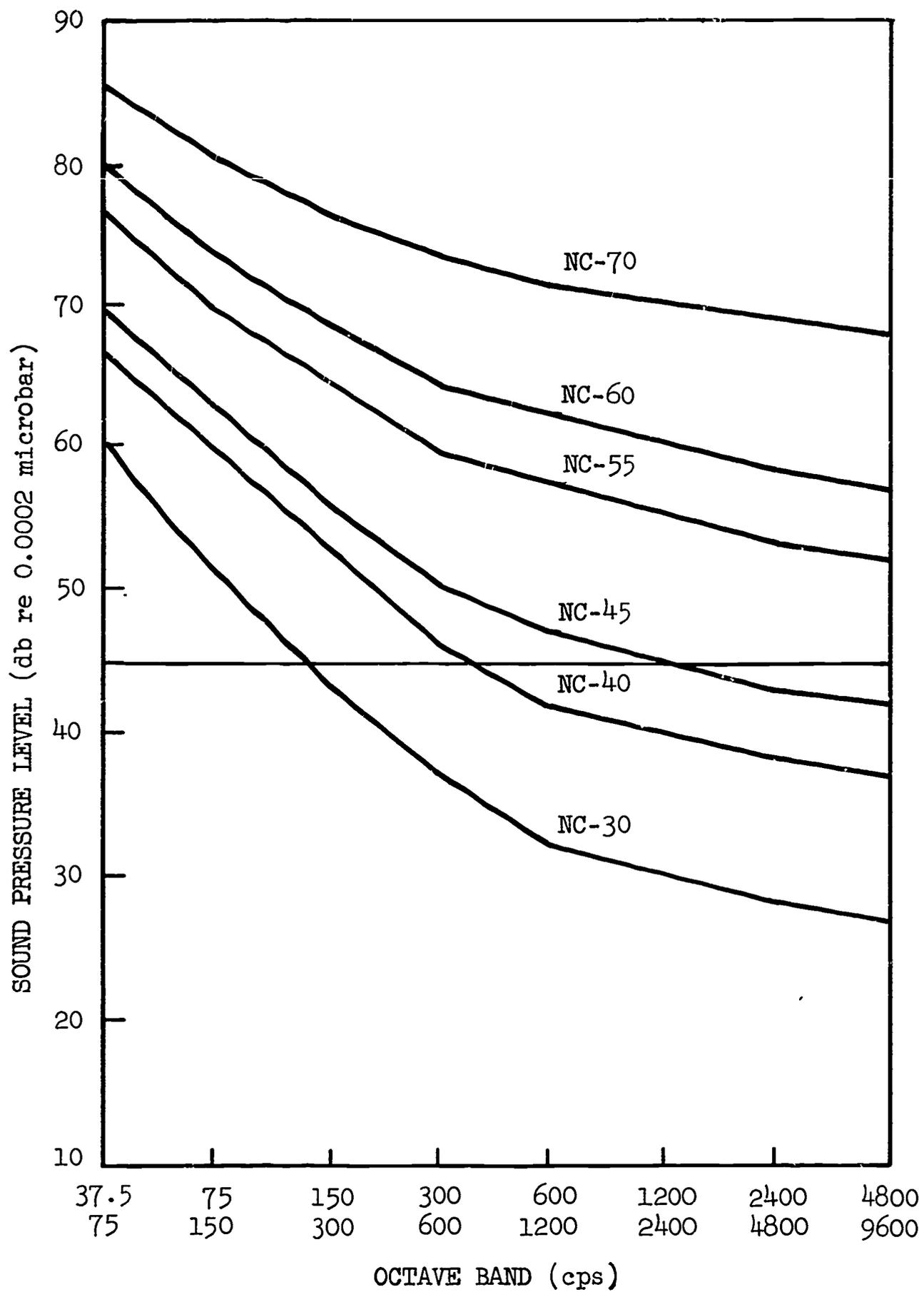
Fig. 2-21 Noise Criteria (NC) Curves for Speech Communication
