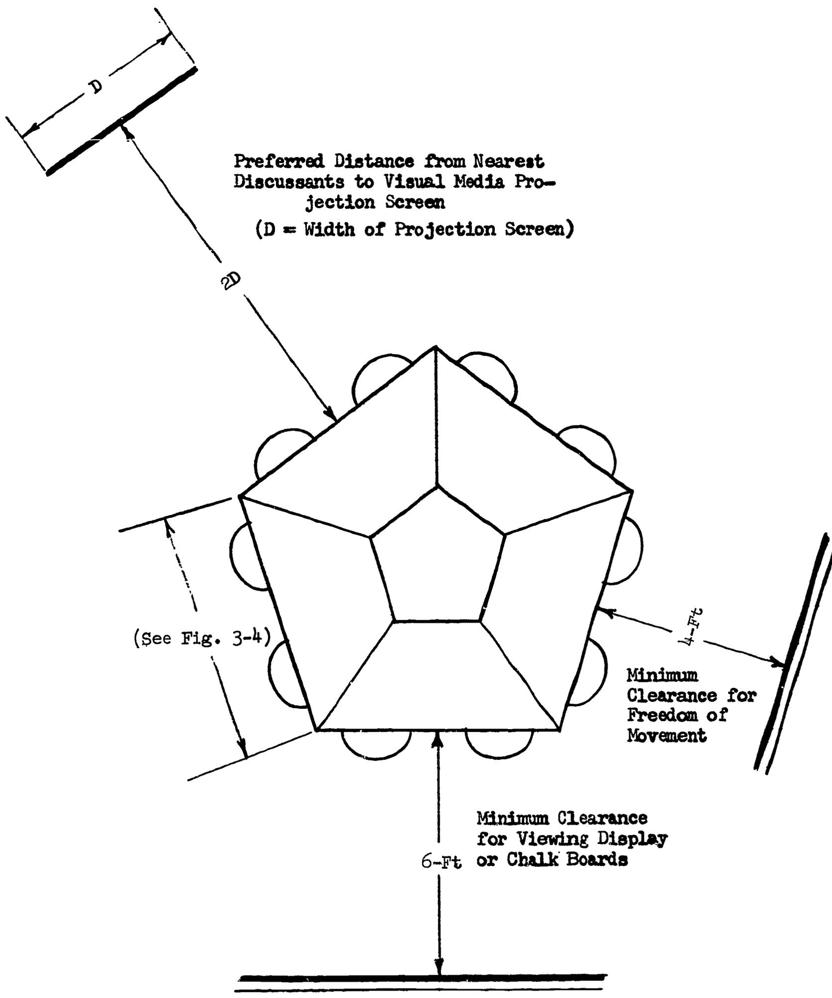
Fig. 3-3 Preferred Clearance Dimensions for Room Layouts
