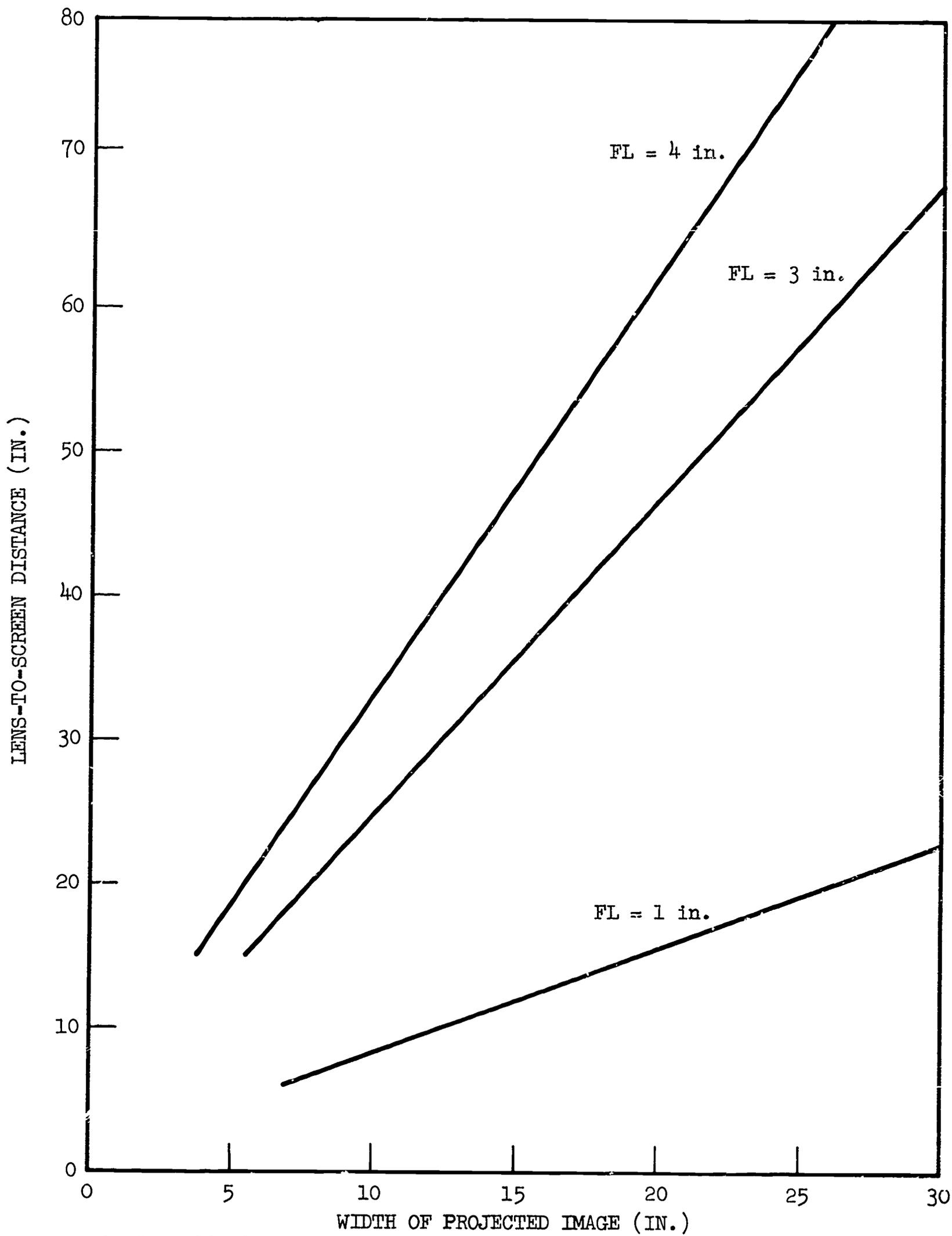
Fig. 2-15 Width of Projected Image of 35-mm Slides as a Function of Lens-to-Screen Distance and Focal Length
