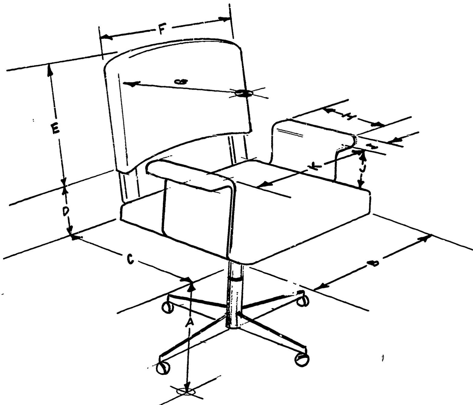
Fig. 2-13 Cushioned Study Chair With Height Adjustment Casters
