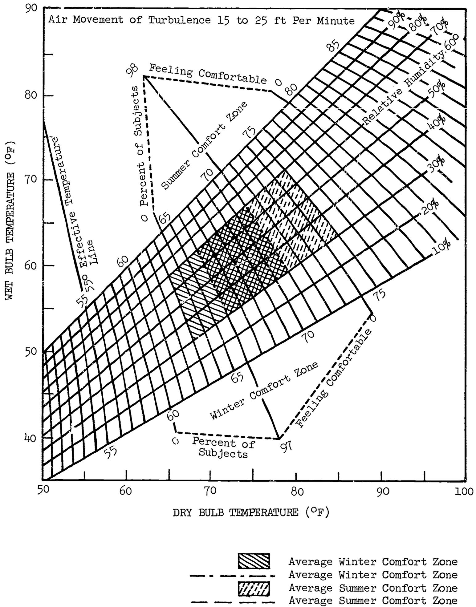
Fig. 2-18 Effective Temperatures for Comfort Requirements
