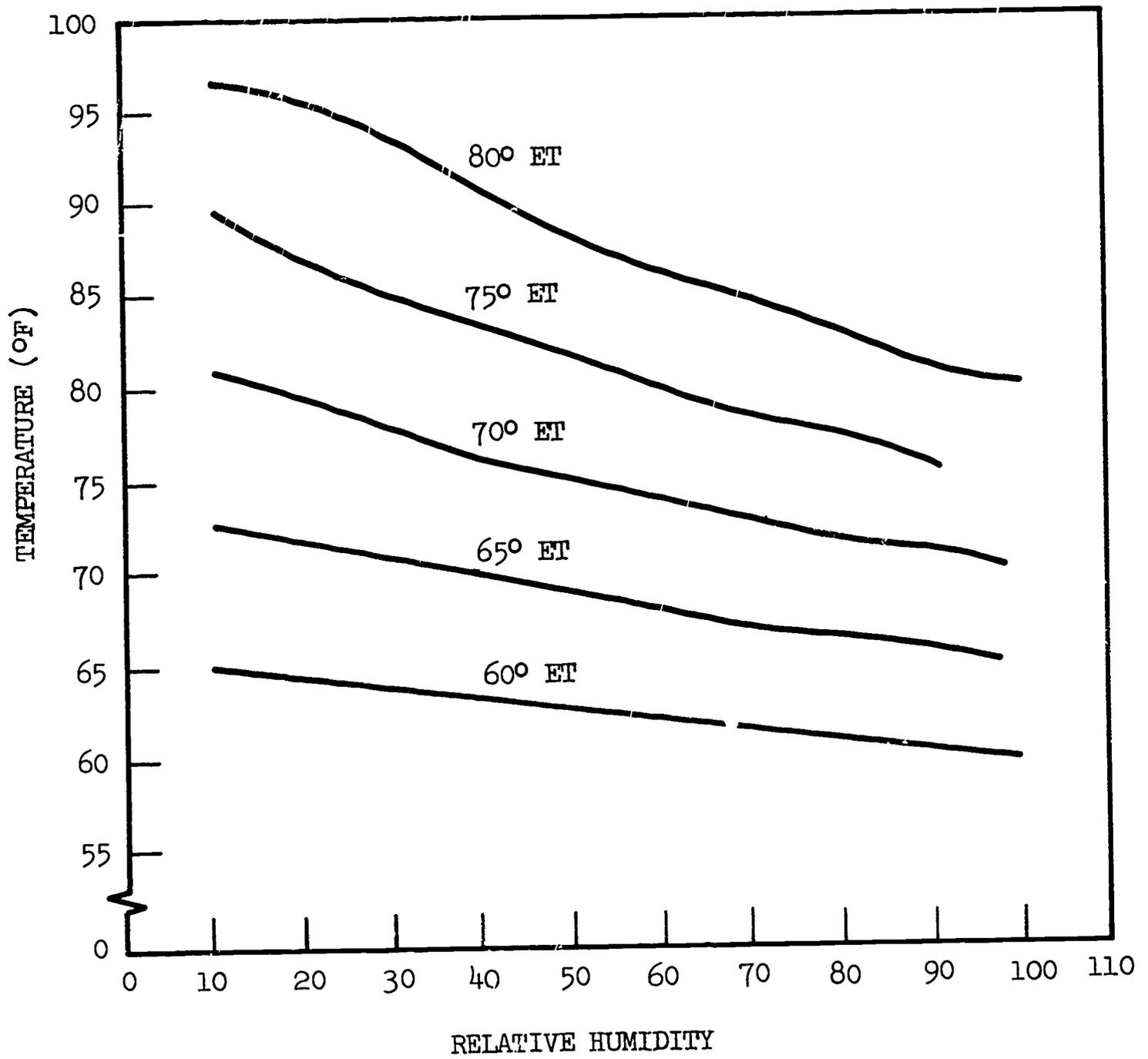
Fig. 2-19 Effective Temperature in Relation to Dry-Bulb Temperature and Relative Humidity
