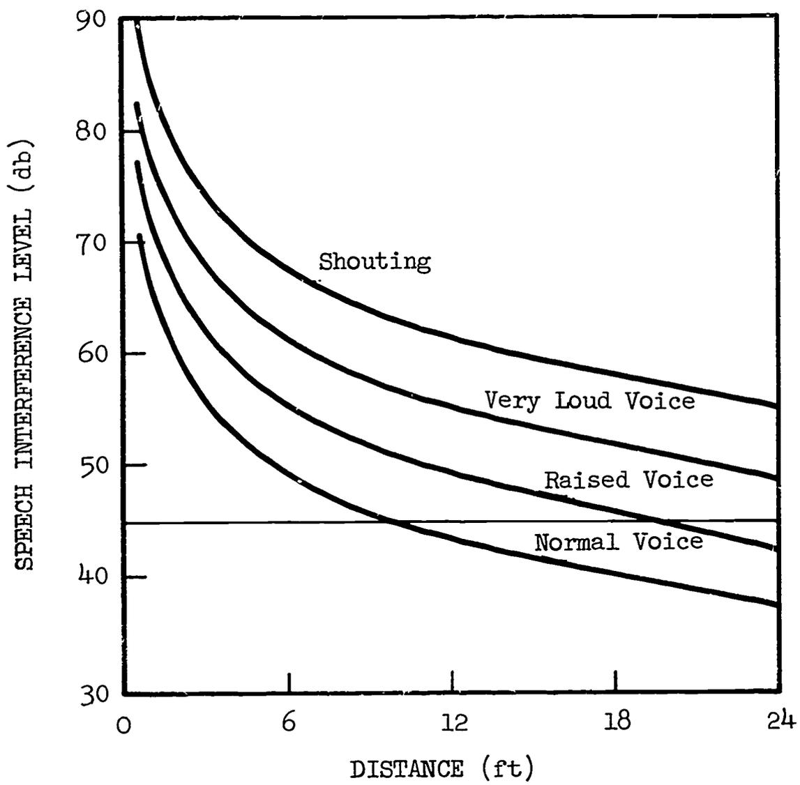
Fig. 2-20 Speech Interference Levels for Various Distances and Voice Levels
