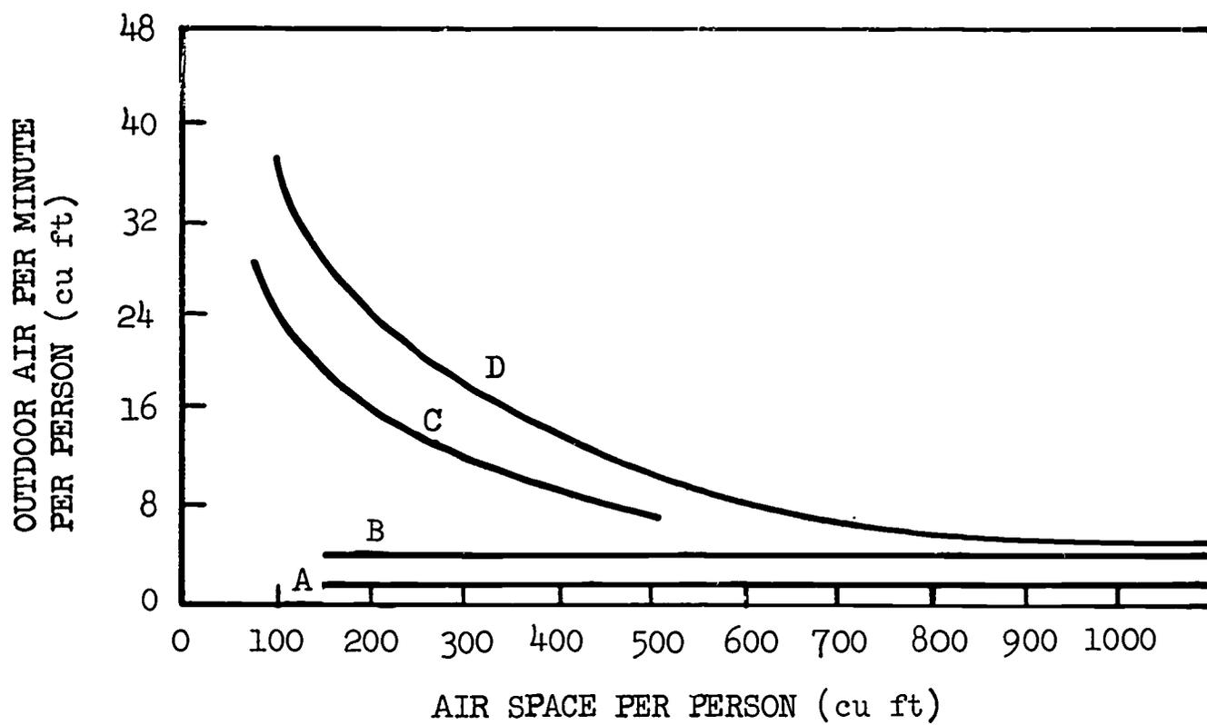
Fig. 2-17 Ventilation Requirements
