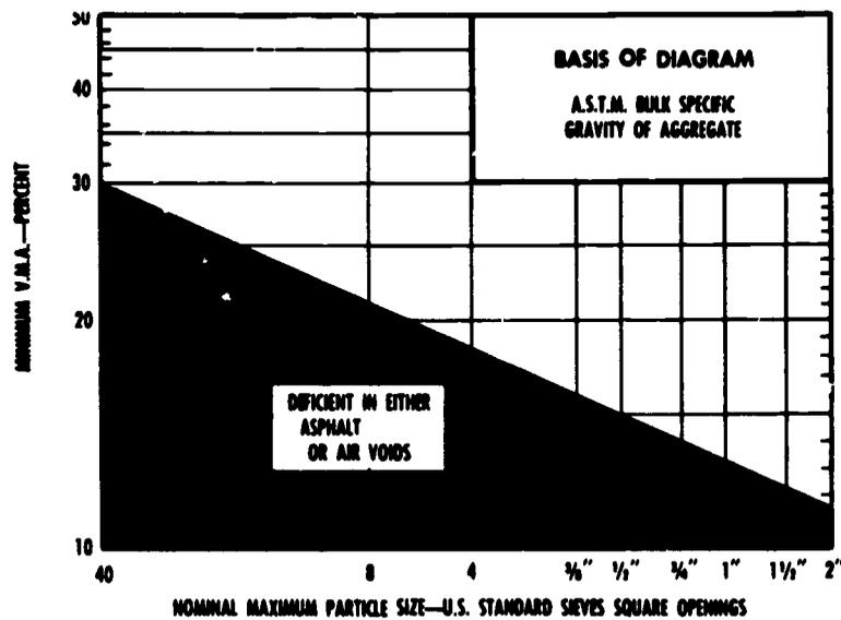
**Figure II-2—Relationship Between Minimum V.M.A. and Nominal Maximum Particle Size of the Aggregate for Compacted Dense-Graded Paving Mixtures**
