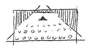
The wasted area is shaded. As a result the teaching area is designed for concentration of visual presentation on two sides of the area. On one is concentrated the audio visual media, including overhead projection over the teachers' head. We had planned E.T.V. likewise, suspended from the ceiling. However, the state E.T.V. allotment is based on one receiver per three (3) classrooms so that these are necessarily on carts to serve each of the areas as needed.
