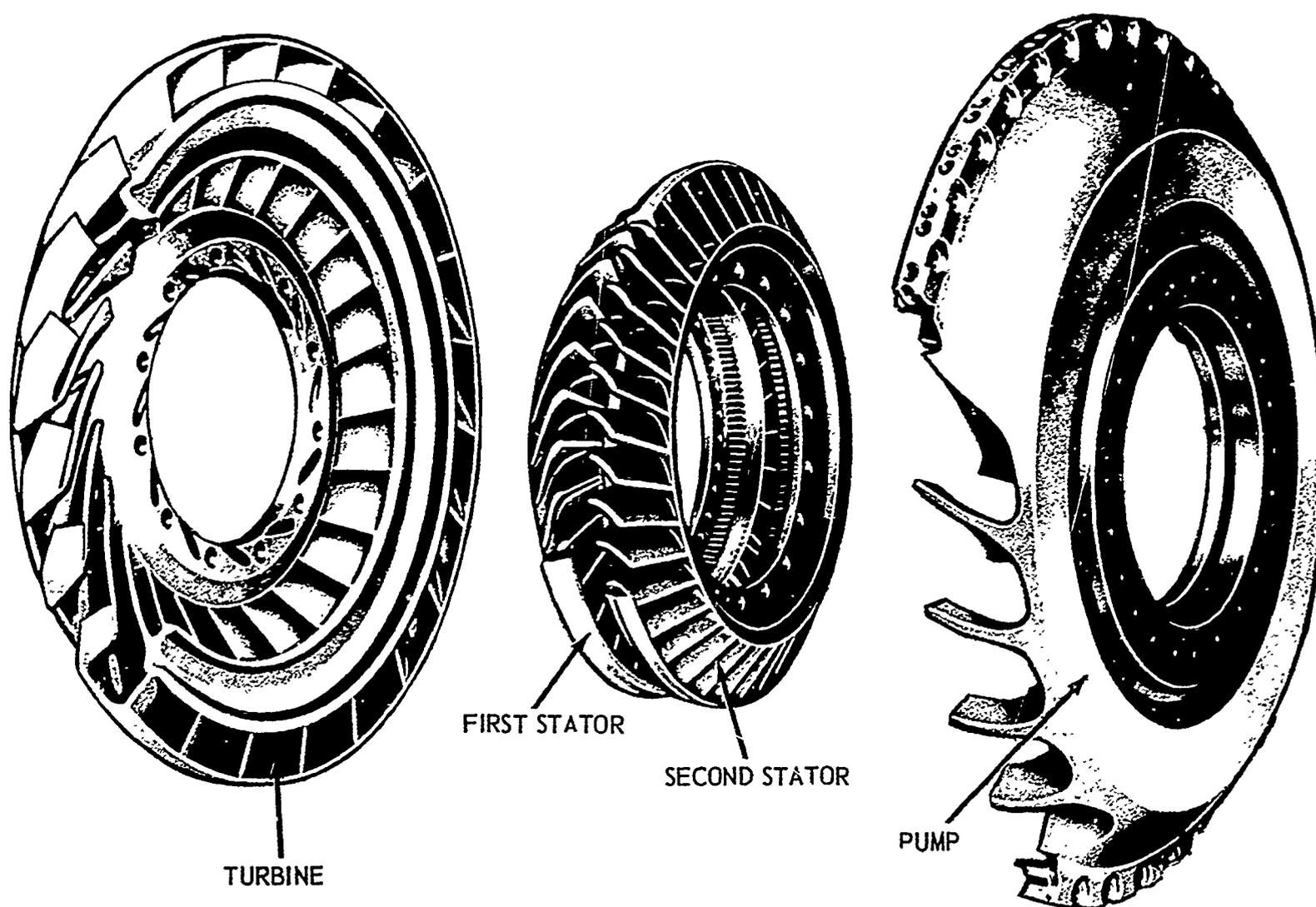
Fig. 16 Four element torquematic converter
