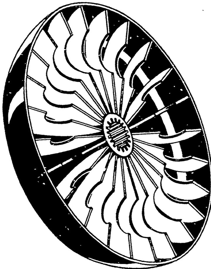
Fig. 3 Fluid coupling pump
