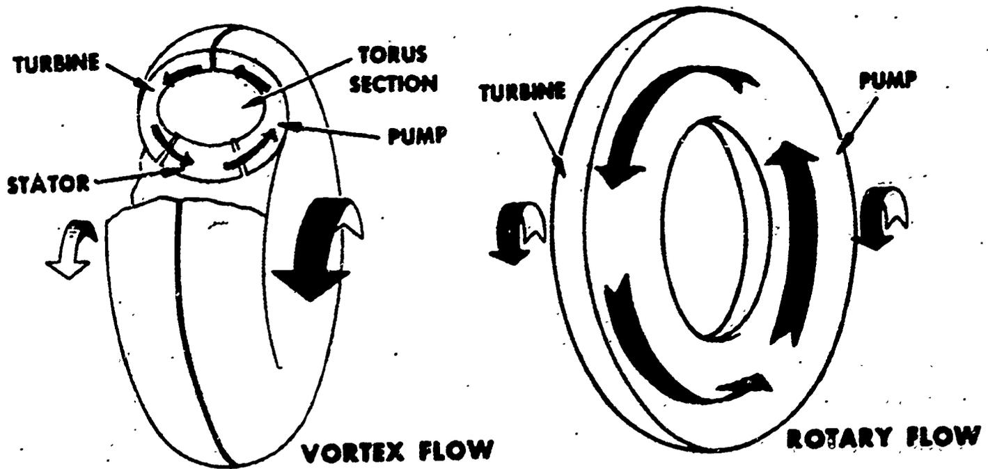
Fig. 11 Oil flow within a converter
