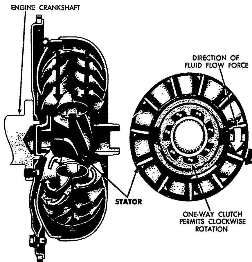
Fig. 15 Converter in fluid coupling phase
