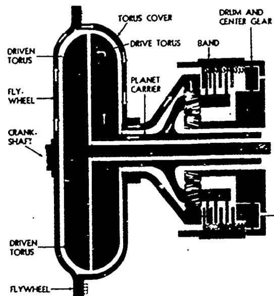
Fig. 6 Hydramatic fluid coupling design
