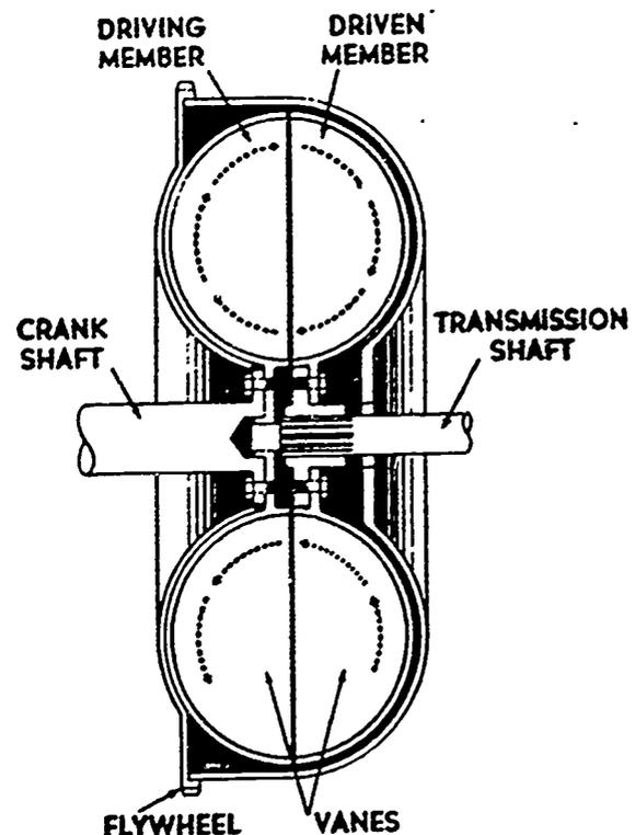
Fig. 1 Cross sectional view of a fluid coupling
