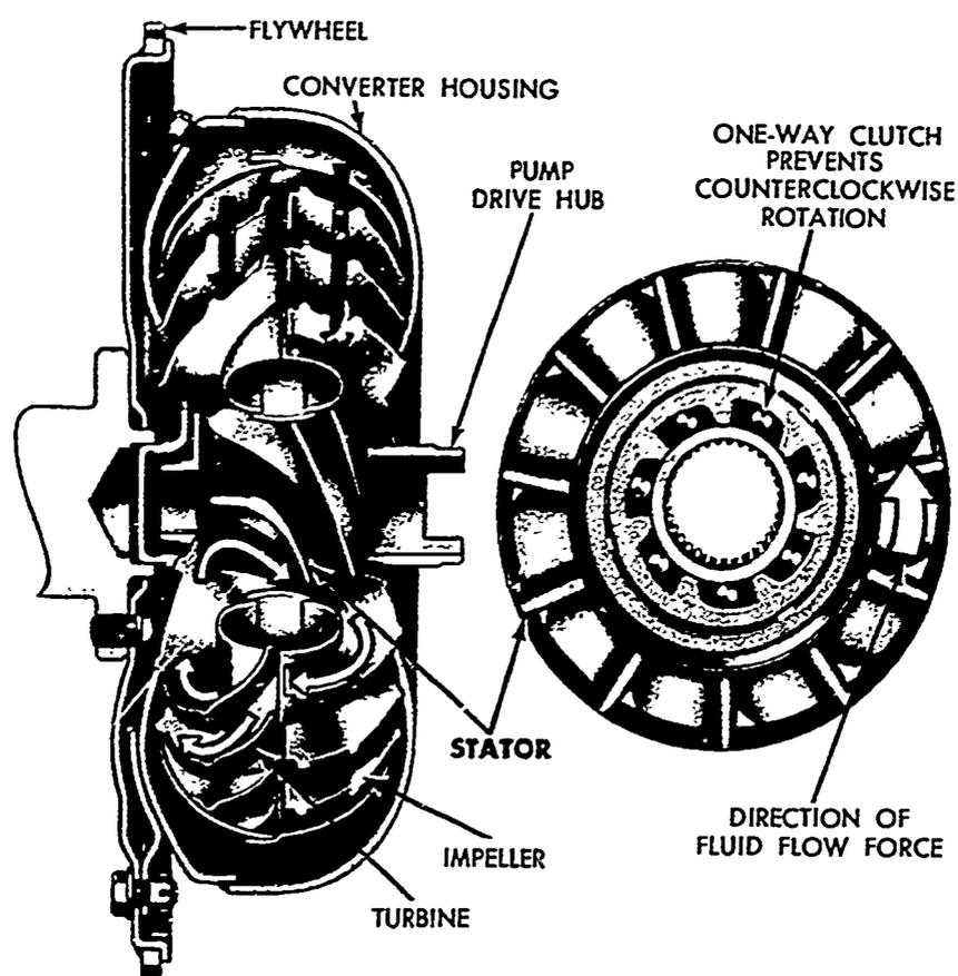
Fig. 14 Converter in torque multiplication phase
