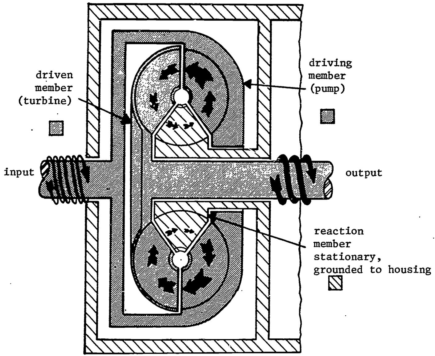
Plate IV Torque converter schematic
