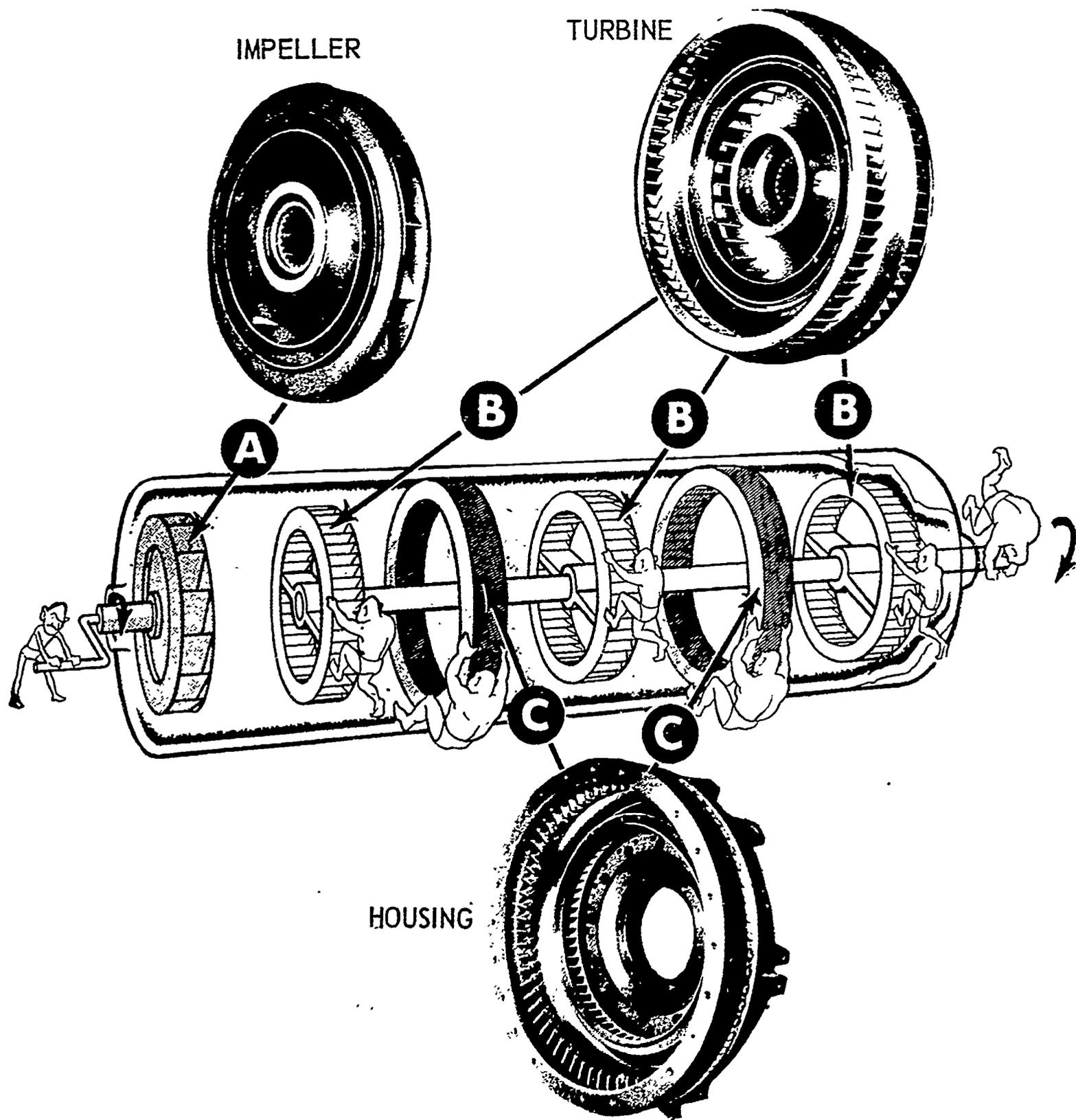
Fig. 18 Operation of a three stage torque converter
