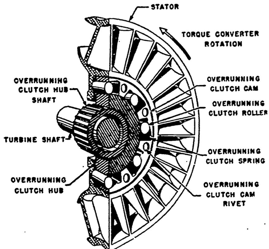
Fig. 12 Roller type stator
