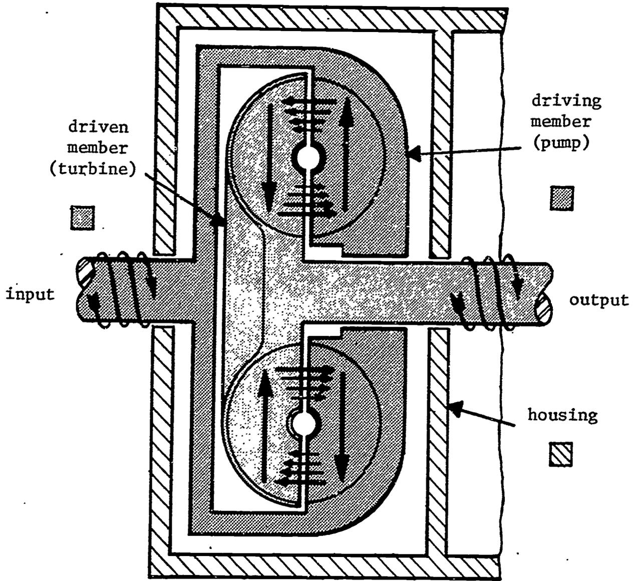
Plate III Fluid coupling schematic
