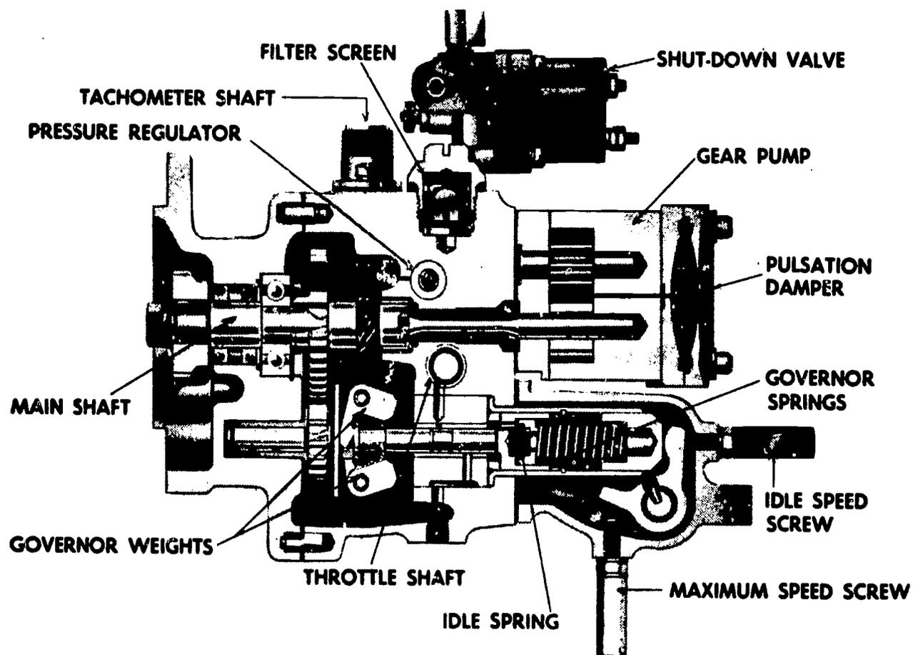
**Fig. 7** PTR fuel pump with variable speed governor.
