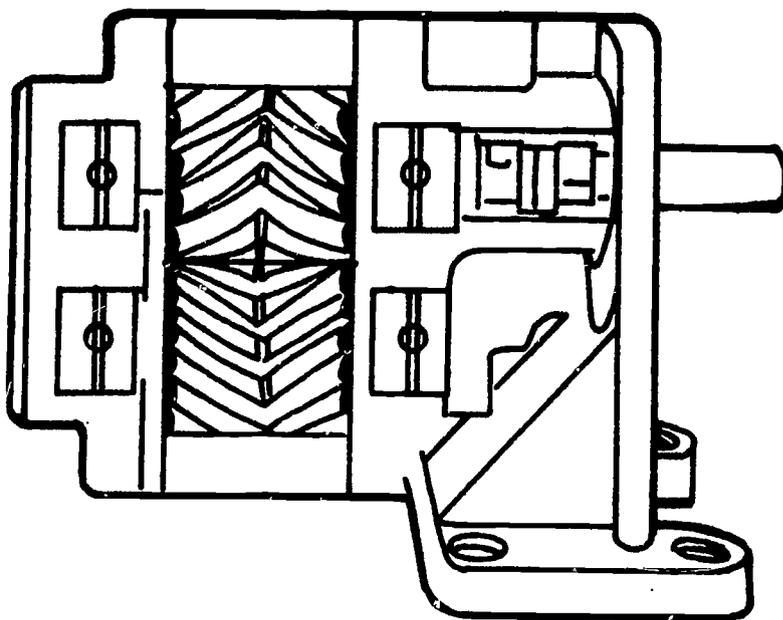
Plate X Herringbone gear pump.
