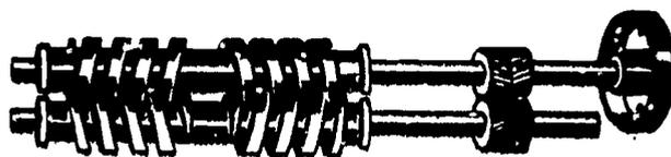
Plate XI Low pitch double-screw pump.
