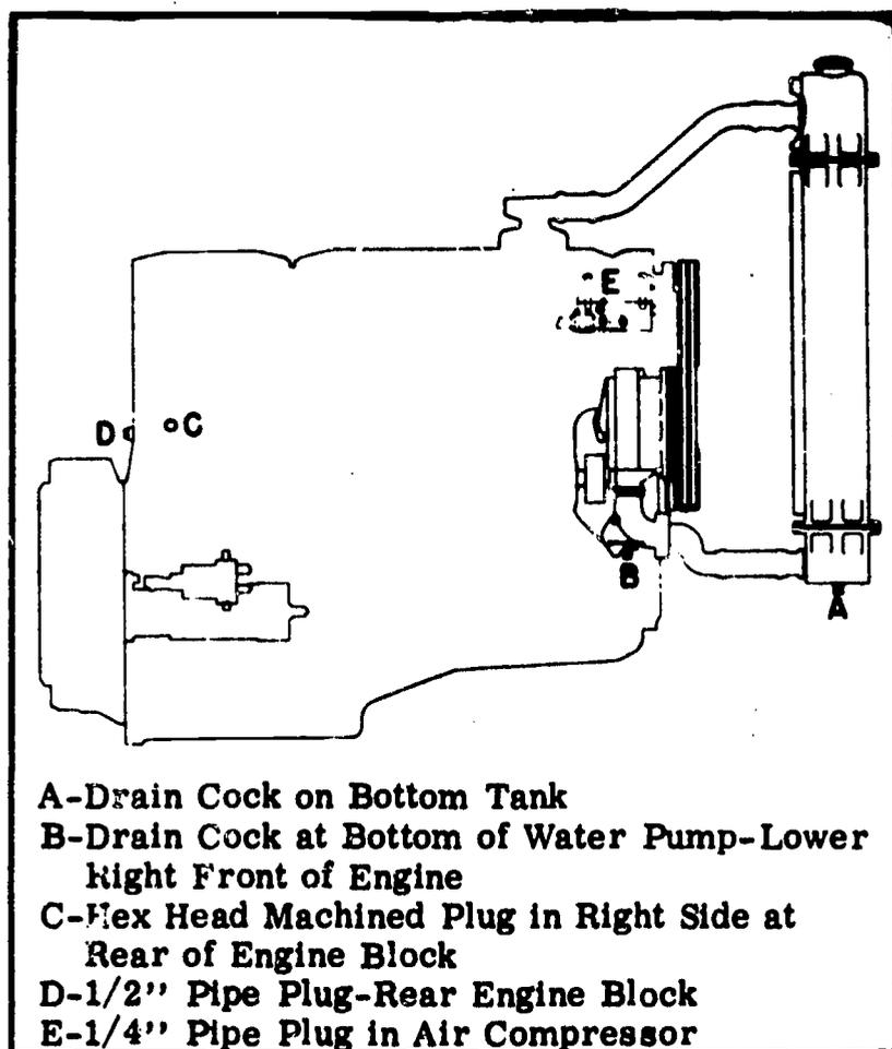
Fig. 12 Typical engine drain points.
