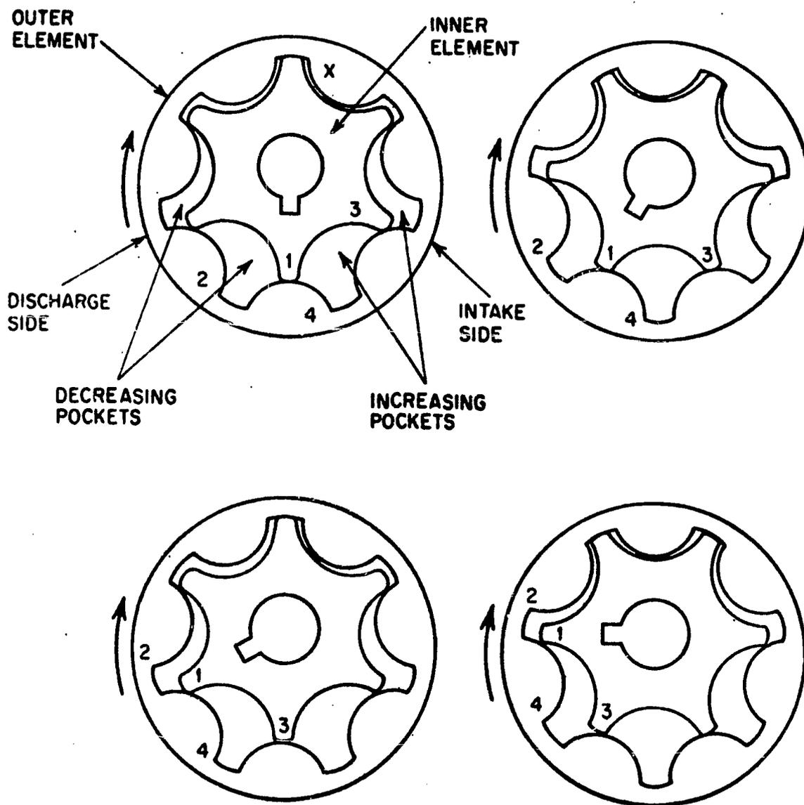
Plate XIV Operation of an internal gear pump.
