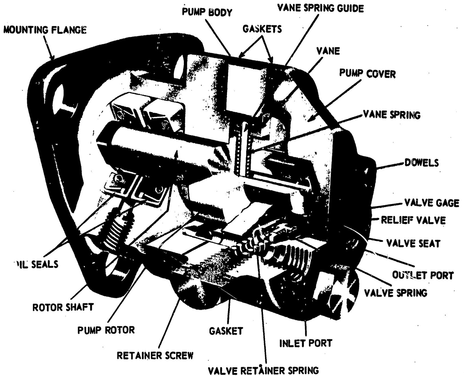
Plate VIII Relief valve in a vane pump.
