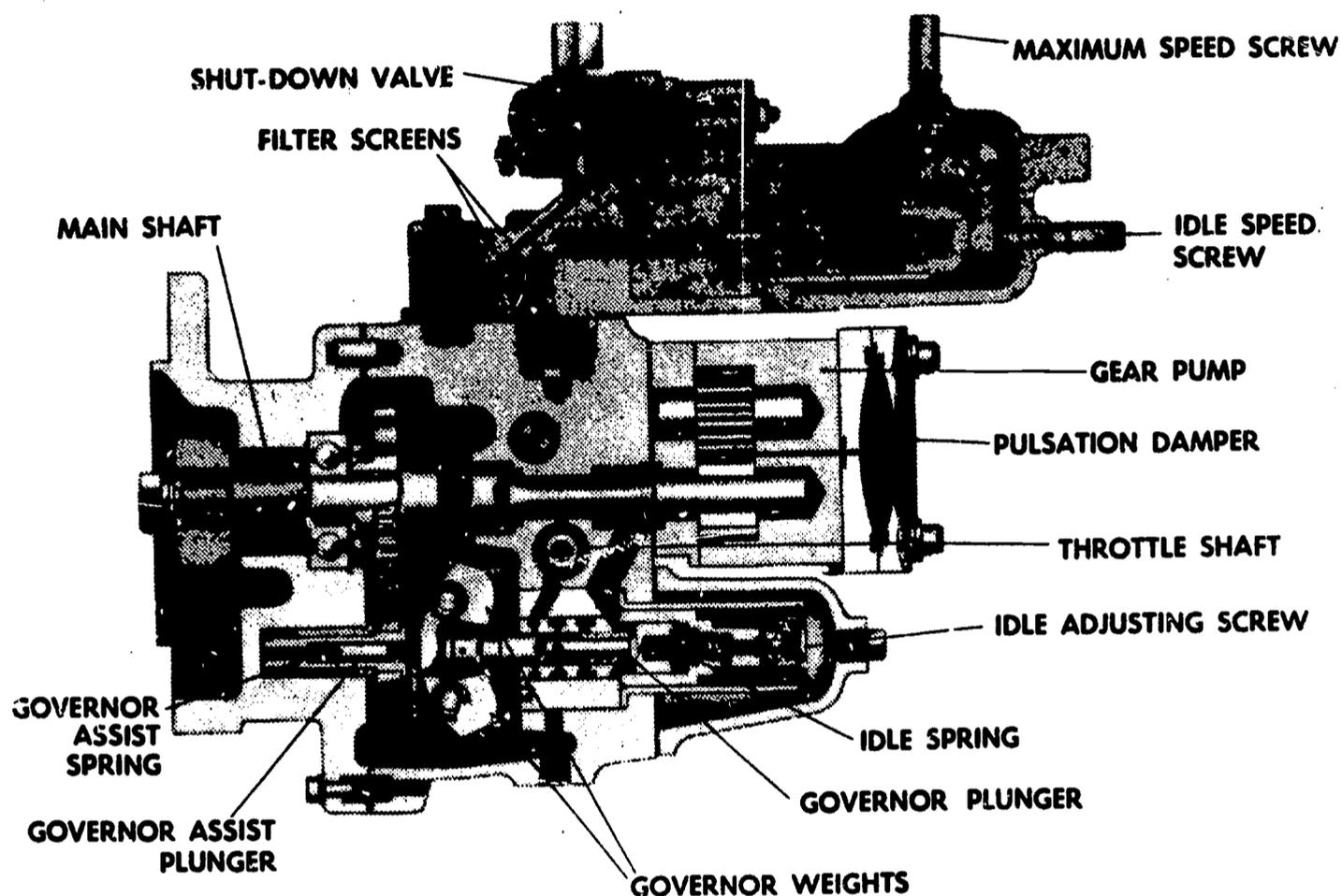
Fig. 8 PTG fuel pump with variable speed governor.
