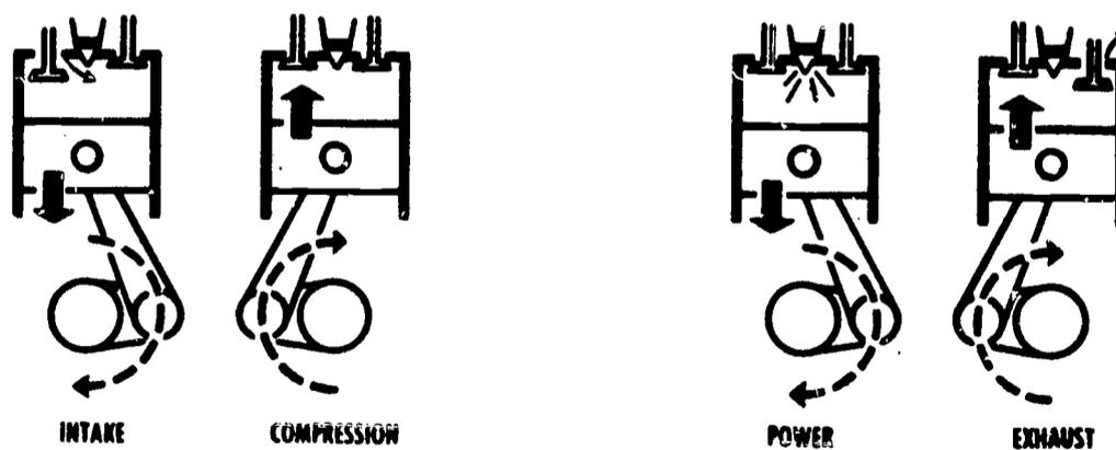
Fig. 2 Four cycle operation.
