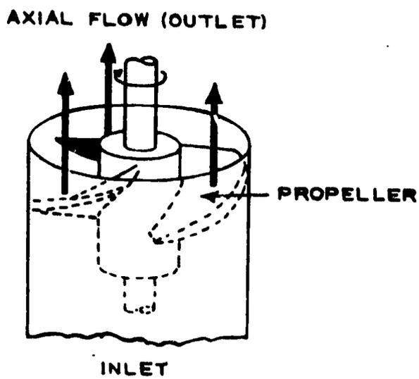
Plate III Propeller pump.
