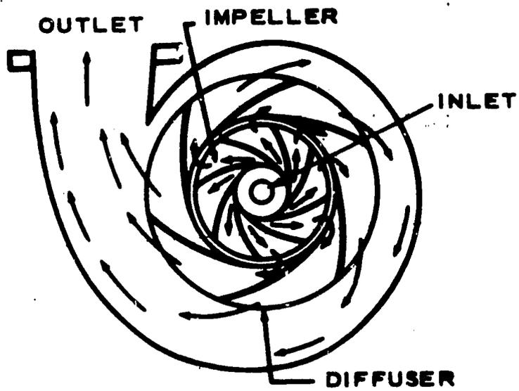
Plate IV Diffuser type of centrifugal pump.
