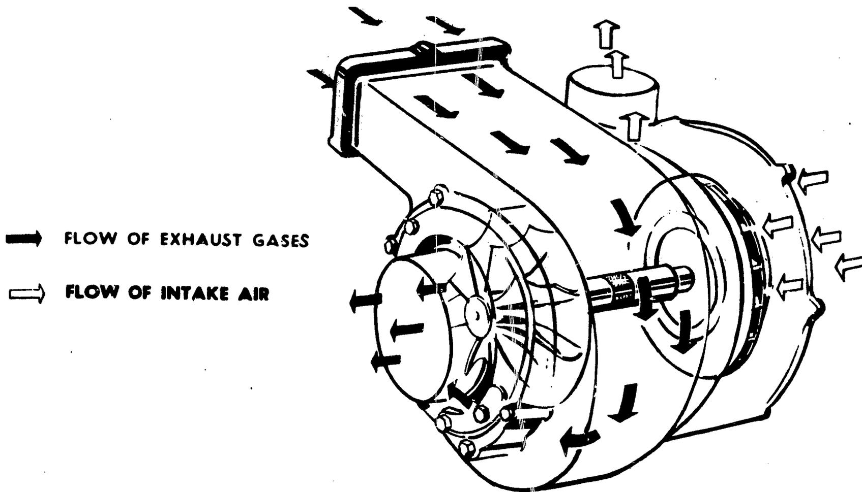
Plate V Cummins turbocharger.
