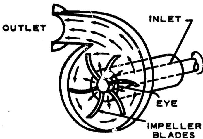
Plate II Volute type of centrifugal pump.
