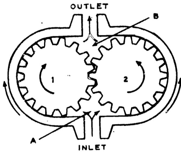
Plate VII Operation of an external gear pump.
