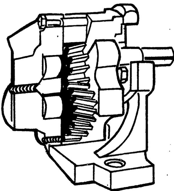
Plate IX Helical gear pump.
