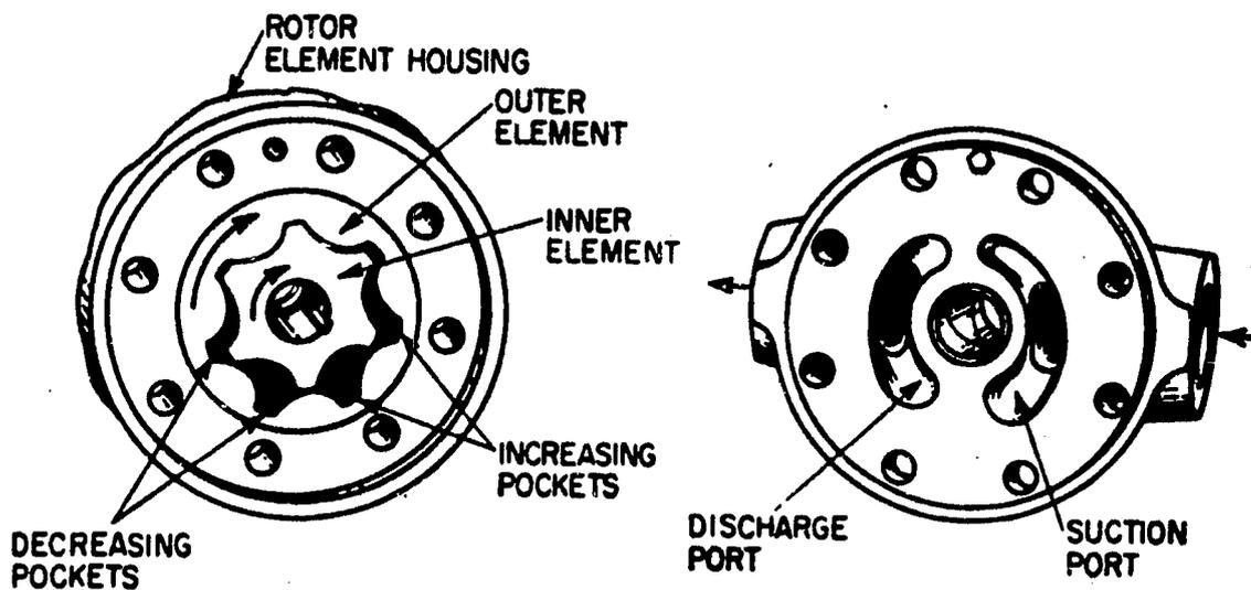
Plate XIII Internal gear pump.
