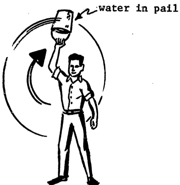
Plate I Centrifugal force holds water in the pail.
