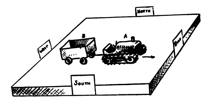
Tractor A is pulling wagon B straight ahead in the direction shown with a force of 100 pounds.
