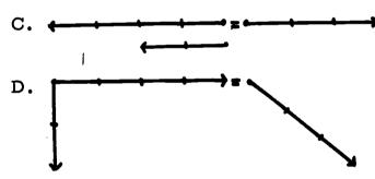
8. If a tractor were hooked to the trailer so that it pulled on the trailer with a force of 100 pounds in a direction opposite to that exerted by the car, which diagram shows the vector subtraction of these forces?
