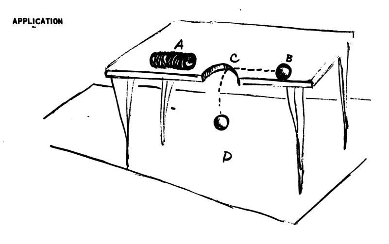
In the picture above, A is an electromagnet which is turned on to attract the steel ball B. The ball is caused to roll toward the magnet but it falls through the hole C in the table, and lands on the floor at D.
