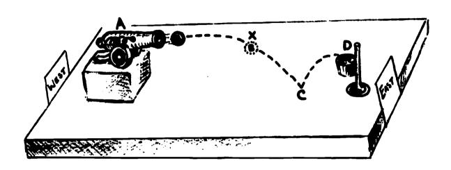
In the picture above, A is a spring cannon that exerts a force of ten pounds on ball B. The ball is shot outward level with the floor. It strikes the floor at C and bounces into the basket D.
