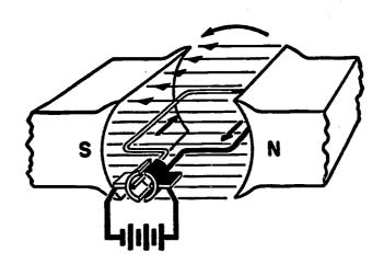
Without magnetism an electric motor would not work. It works because of the reaction of the magnetic field of the armature to the magnetic field of the field coil. The field coil is the fixed part of the electric motor and the armature is the part that turns.
