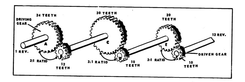
The picture shows six spur gears mounted on four shafts. The number of teeth in each spur gear is shown. Also shown are the speed ratios for the various pairs of gears.
