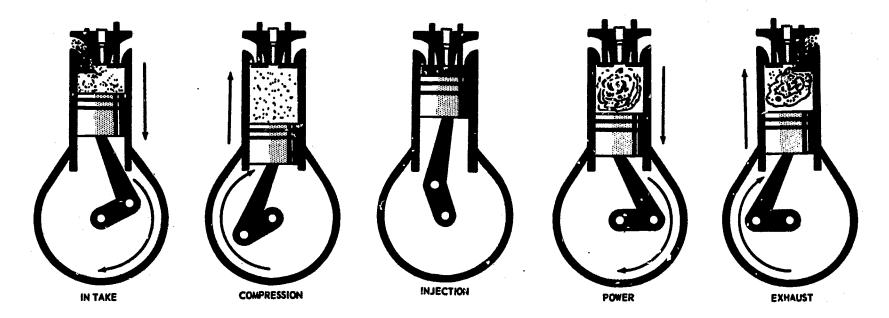
These drawings show the operation of a four-cycle diesel engine. The four strokes (or cycles) are the intake stroke, the compression stroke, the power stroke, and the exhaust stroke. These are very much like the four strokes of a four-cycle gasoline engine.
