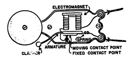
Most simple foor bells are made very much like the picture here. They all have an electromagnet, an armature with a clapper attached, and a con act point.
