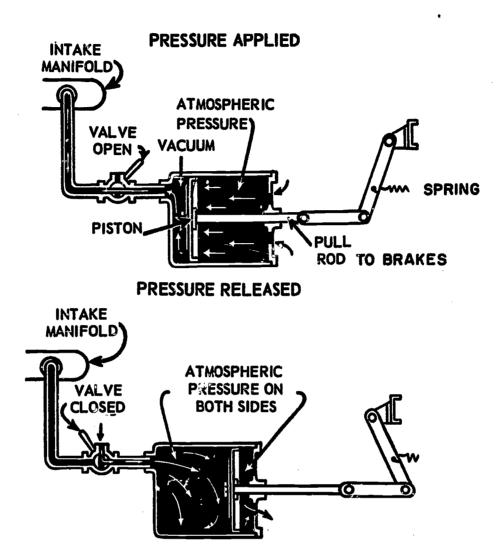
The vacuum power system is used to operate power brakes on automobiles and trucks. These diagrams show how it operates. The vacuum power cylinder contains a piston. The piston is connected to a pull rod which operates the brakes.
