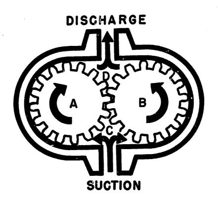
This is a rotary pump. Gears A and B rotate in opposite directions. Gear A is driven by a power source and gear B turns freely. Liquid enters the pump at the bottom and is carried up to the discharge in the small spaces formed between the gear teeth and the wall of the pump chamber.
