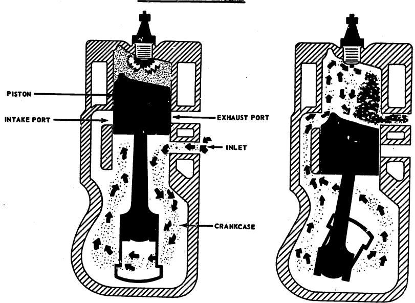
This diagram shows how one type of two-cycle gasoline engine works. The two-cycle engine needs only two piston strokes instead of four like most automobile engines. Two-cycle gasoline engines are used for outboard motors, lawn mowers, lightweight motor-cycles, etc.
