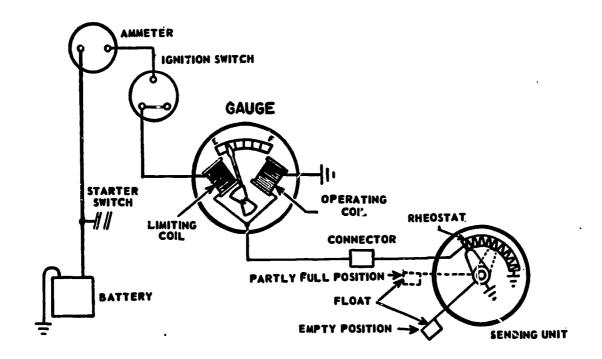
The amount of gasoline in the gas tank of an automobile is shown by the fuel gauge. There are many types of fuel gauges. One of the most common is the coil type shown here. It is an electrical fuel gauge and usually works only when t ignition switch is on. You can see the ignition switch in the diagram. The power comes from the battery.
