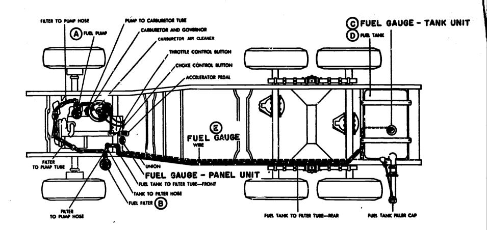
This diagram shows the fuel system for a six-wheel truck. It is very similar to the fuel system on most gasoline-driven vehicles.
