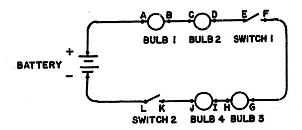
This is a diagram of an electric circuit. When the two switches are closed, the electric current goes from one terminal of the battery and flows through the wires, bulbs, and switches (through points A, B, C, D, E, F, G, H, I, J, K, and L, in turn) back to the other terminal of the battery. Current will not flow if either of the switches is open. The switches are shown open in the diagram.
