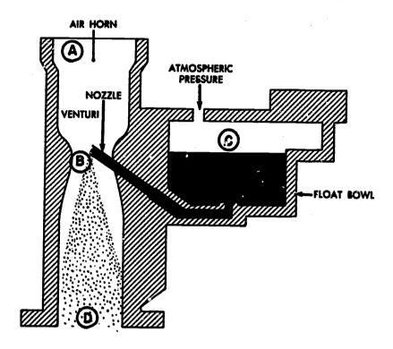
A carburetor is one of the essential parts of a gasoline engine. The drawing shows a greatly simplified carburetor. Only the basic parts are shown.
