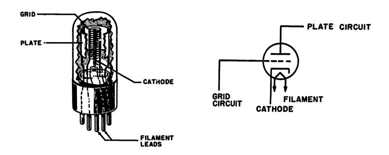
The vacuum tube pictured here is called a triode. The cutaway drawing shows how the parts actually look. The diagram shows how the parts work.
