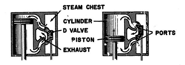
This is a diagram of the steam chest, cylinder, piston, and D valve of a railroad locomotive. Steam under high pressure goes from the boiler to the steam chest. From the steam chest it is fed alternately through the two small openings, called ports, into the cylinder. The upper port is open in the left-hand diagram.
