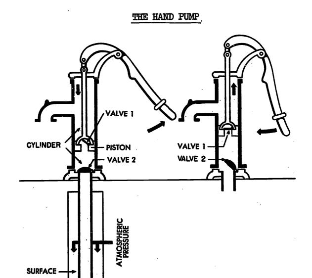
The diagram shows a hand pump for pumping water from a well. It raises water by producing a partial vacuum in the pipe to the well. A partial vacuum means that the air or water pressure inside the pipe is less than that of the air outside. The atmospheric pressure forces the water up the pipe by pressing down on the surface of the water in the well.
