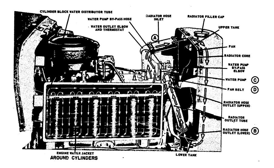
Most automobile engines use a liquid system like the one shown here. A cooling system carries away the heat of combustion from the cylinders.
