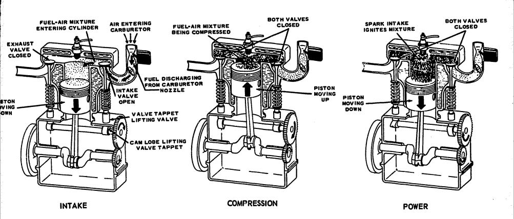
The drawings show the four strokes in a four-cycle gasoline engine. The intake stroke brings the air-and-fuel mixture into the cylinder. The piston moves down and the intake valve opens. Air entering the carburetor mixes with fuel coming from the carburetor nozzle. This mixture goes into the cylinder through the open intake valve.
