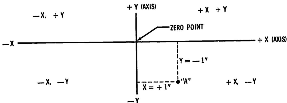
Fig. 9—3. Standard Cartesian coordinate system
