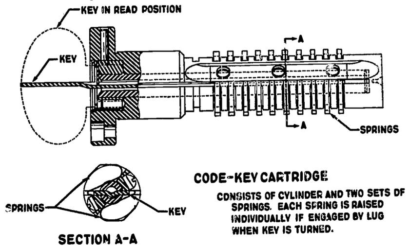
Fig. 4-18. N/C preset tool key cartridge
