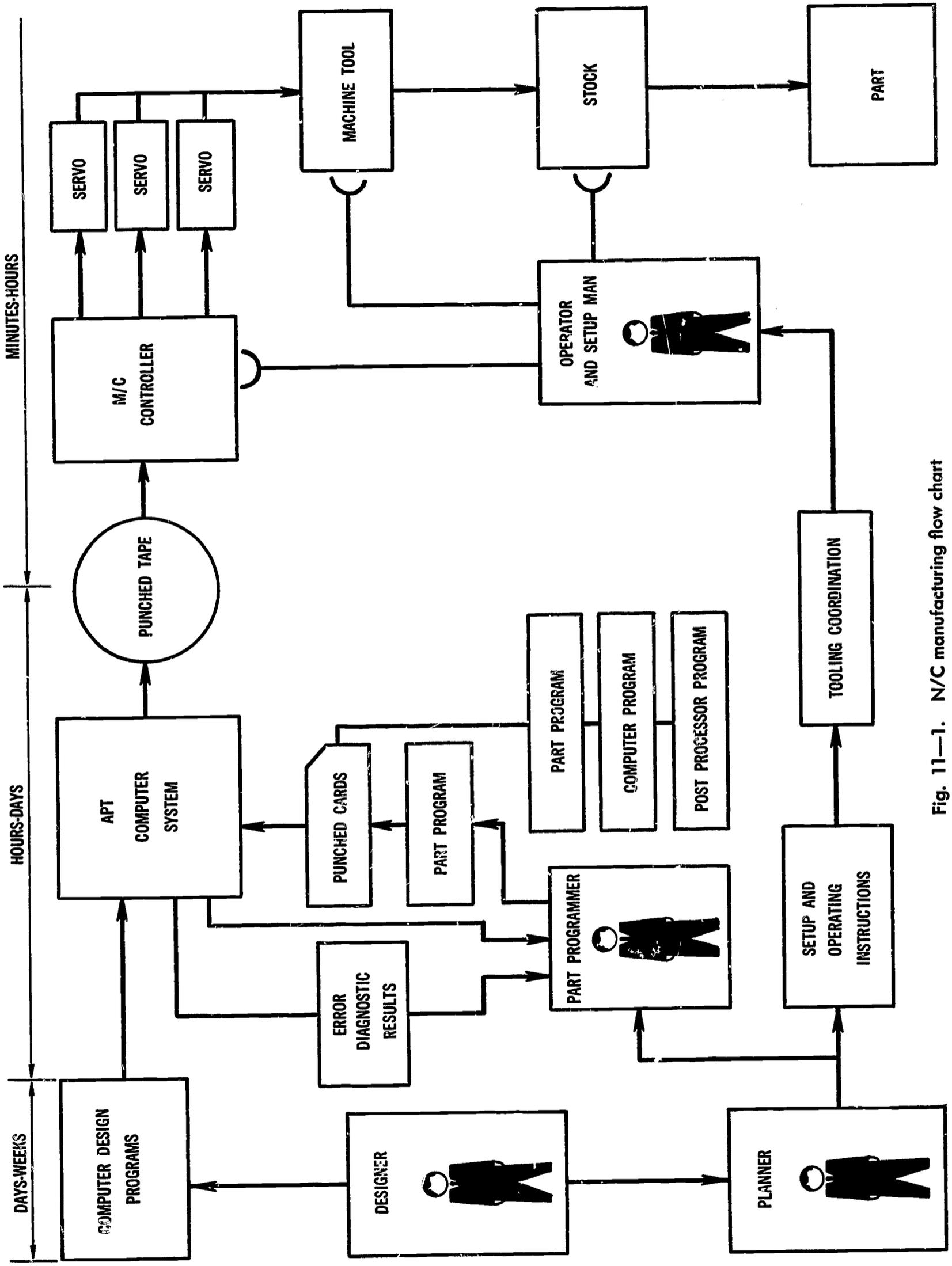
Fig. 11-1. N/C manufacturing flow chart
