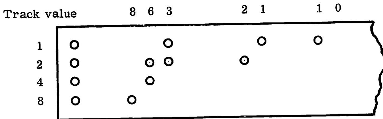
Fig. 8-1. Four-track binary tape
