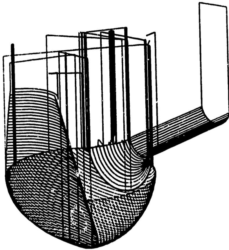
*THIS DEMONSTRATION PROGRAM DEPICTS THE TOOL PATH AUTOMATICALLY GENERATED BY AUTOPROMPT TO CUT A PART COMPOSED OF TOROIDAL AND PLANE SURFACES*
