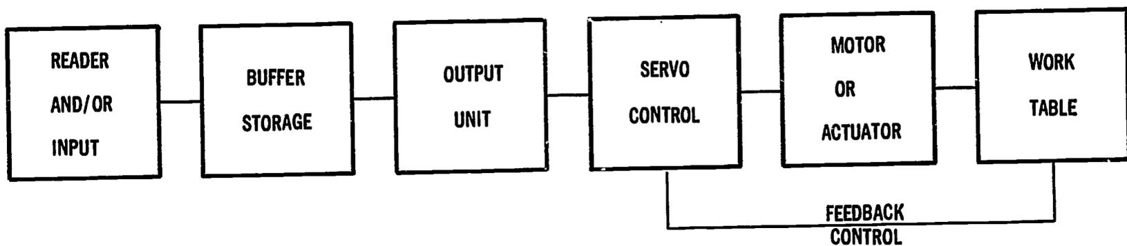
Fig. 3—1. Block diagram of control system with feedback
