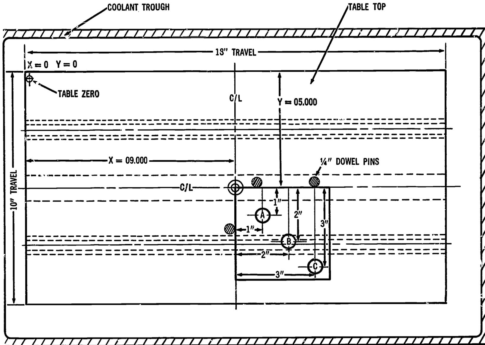
Fig. 10—4. Sample N/C drawing of part on machine table
