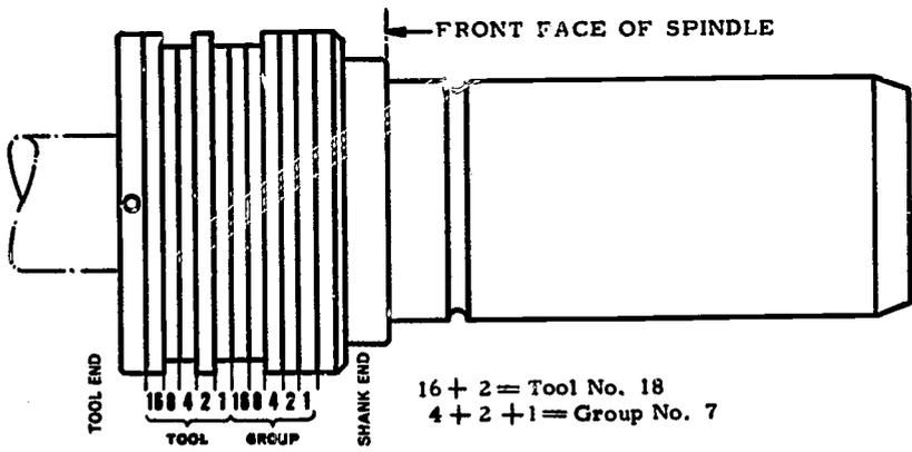
Fig. 4-15. Coding rings, Milwaukee-Matic tool holders
