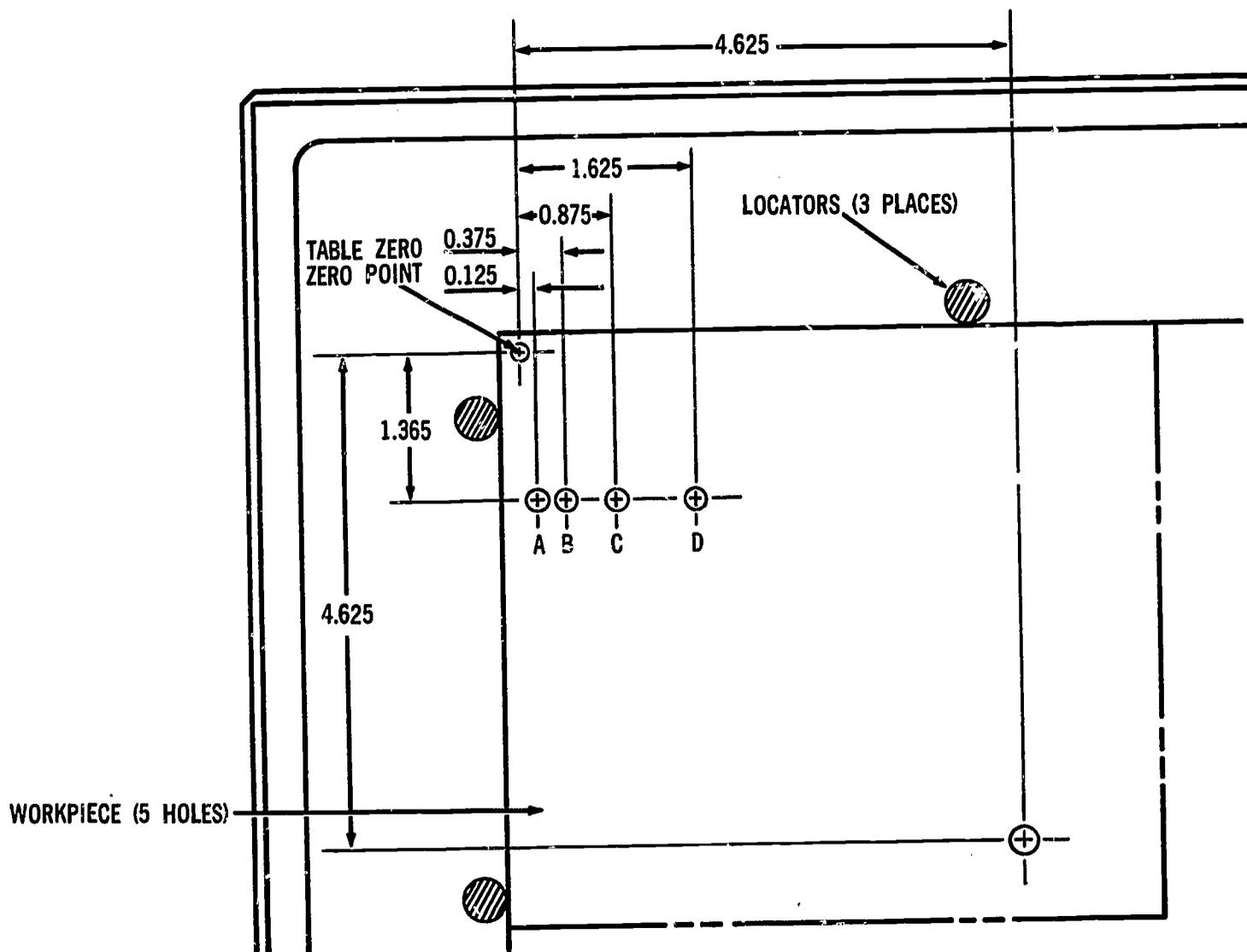
Fig. 10—3. Sample N/C drawing
