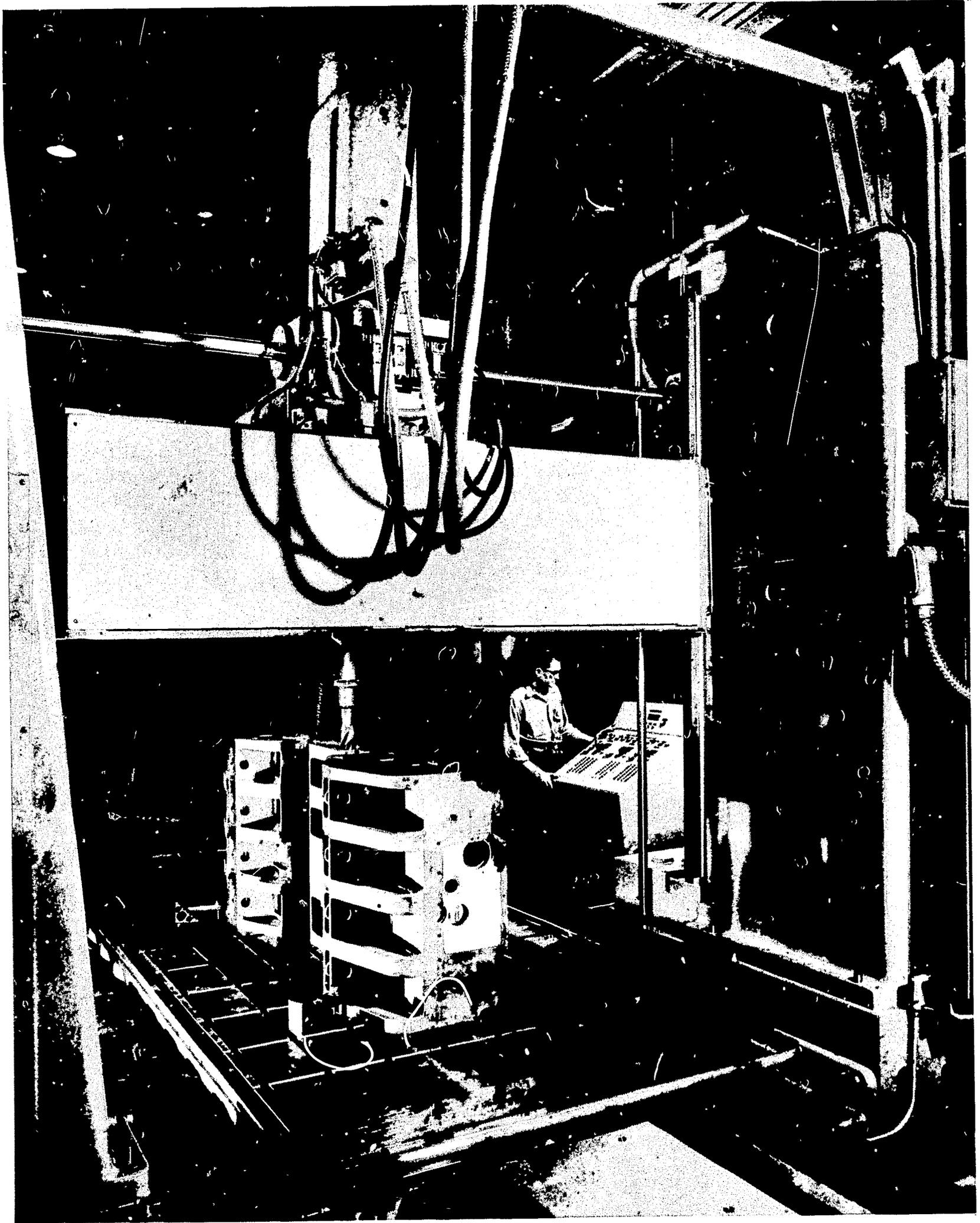
Fig. 2—5. A numerically controlled rail-type machine tool with remote operator control console
