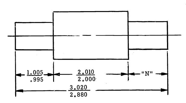
Compute the limits of factor "N" when the overall dimension of the object is at maximum and minimum material conditions.
